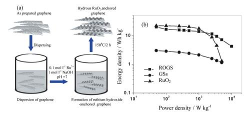
Fig. 7 (a) The preparation scheme of RuO<sub>2</sub>/GSs composites (ROGS) and (b) Ragone plot for the as-prepared GSs, RuO<sub>2</sub>, and ROGS (Ru, 38.3 wt%) (modified from ref. 59a)
