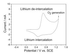
Fig. 18 CV curve of in LiNi<sub>1/3</sub>Co<sub>1/3</sub>Mn<sub>1/3</sub>O<sub>2</sub> in 2 mol  $I^{-1}$  Li<sub>2</sub>SO<sub>4</sub> aqueous solution (modified from ref. 108).
