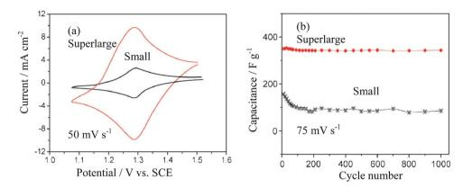
Fig. 13 (a) Typical CV curves and (b) cycling performance of super-large PbO<sub>2</sub> dendrites composed of trigonal nanoplates and the small dendrites in 5.0 mol  $I^{-1}$  H<sub>2</sub>SO<sub>4</sub> solution recorded a scan rate of 75 mV s<sup>-1</sup> (modified from ref. 82c).
