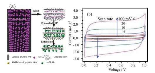
Fig. 11 (a) Illustration of the formation of the composite of  $\alpha$ -MoO<sub>3</sub>-decorated graphene sheets by electrolytic exfoliation from graphite with the assistance of molybdate and (b) CV curves of the composite in 6 mol l<sup>-1</sup> KOH (modified from ref. 49a).
