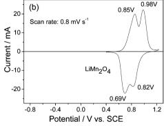
Fig. 17 (a) SEM micrograph of the porous LiMn<sub>2</sub>O<sub>4</sub> and (b) CV curve of the micrometer LiMn<sub>2</sub>O<sub>4</sub> in the saturated Li<sub>2</sub>SO<sub>4</sub> solution (modified from ref. 10b and 104).
