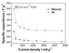
Fig. 6 (a) CV curves of an AC in 6 mol l<sup>-1</sup> KOH aqueous electrolyte and (b) comparison of gravimetric capacitances against current density for the AC and the commercial Maxsorb carbon (modified from ref. 51b).
