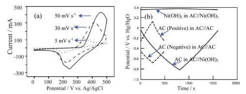
Fig. 15 (a) CV curve of Ni(OH)<sub>2</sub> in alkaline solution and (b) charge/discharge curves of the positive and negative electrodes in the AC//Ni(OH)<sub>2</sub> ASC and electric double layer capacitors of AC//AC at 1 mA cm<sup>-2</sup> in 10 mol  $I^{-1}$  KOH agueous solution (modified from ref. 87b and 90c).
