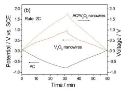
Fig. 12 (a) CV curve of  $V_2O_5$  nanowires and Ni mesh (current collector) and (b) charge/discharge curves of AC// $V_2O_5$  nanowires in 0.5 mol  $I^{-1}$   $K_2SO_4$  aqueous solution (modified from ref. 6a).
