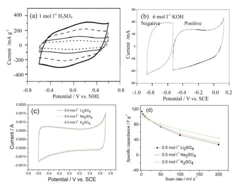
Fig. 2 CV curves of AC as negative electrodes in different aqueous electrolytes: (a), (b) (modified from ref. 12b), (c) 0.5 mol l<sup>-1</sup> Li<sub>2</sub>SO<sub>4</sub>, Na<sub>2</sub>SO<sub>4</sub> and K<sub>2</sub>SO<sub>4</sub> solutions and (d) the change of capacitance with the scan rate in different aqueous electrolytes (modified from ref. 13). Note: Fig. 2b also shows that AC can also be positive electrodes
