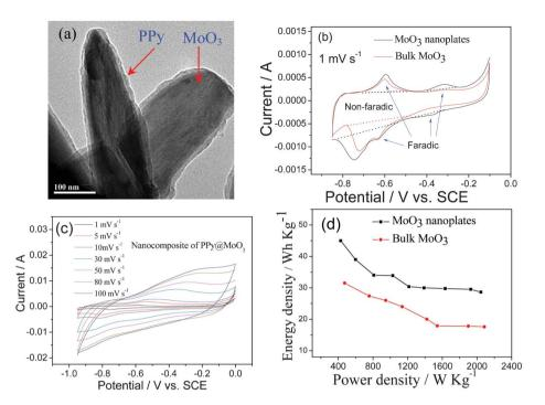
Fig. 4 (a) TEM micrograph of PPy coated MoO<sub>3</sub> nanorods, (b) CV curves of the bulk and nanoplates MoO<sub>3</sub>, (c) CV curves of the PPy@MoO<sub>3</sub> nanocomposite at different scan rate and (d) Ragonne plot of the ASCs based on MoO<sub>3</sub>//AC in 0.5 mol  $I^{-1}$  Li<sub>2</sub>SO<sub>4</sub> solution (modified from ref. 6c and 49c).
