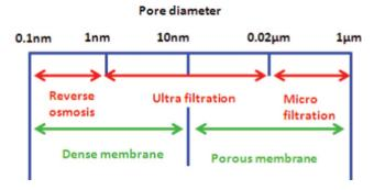
Fig. 2 Filtration spectrum; micro-, ultra-filtration and reverse osmosis.
