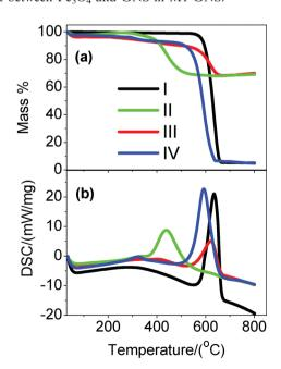
Fig. 5 (a) TG and (b) DSC curves of (I) GNS, (II) M1-GNS, (III) M2-GNS, and (IV) graphene sheets obtained from M1-GNS after removing the Fe<sub>3</sub>O<sub>4</sub> using HCl (1 mol/L).
