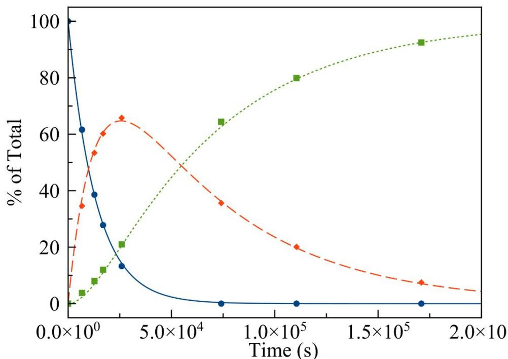
Fig. 5. Representative concentration vs time data for the axial ligand substitution of  $[\text{Co}(\text{3F-salen})(\text{3F-BnNH}_2)_2]^+$  with MeIm at 37 °C. Concentrations of species (A) (solid blue line, circular marker), (B) (broad dashed orange line, diamond marker), and (C) (short dashed green line, square marker) were fit to equations 1, 2, and 3, respectively. Here, (A), (B), and (C) refer to ligand substitution reactants and products shown in Fig. 4.
