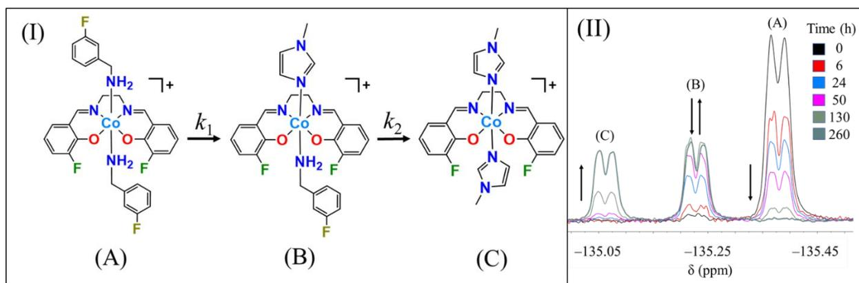
Fig. 4. Panel I: Proposed ligand exchange pathway of  $[\text{Co}(\text{Schiff base})(\text{L})_2]^+$  complexes by MeIm. Panel II: <sup>19</sup>F NMR spectra of  $[\text{Co}(3\text{F-salen})(3\text{F-BnNH}_2)_2]^+$  over time. Chemical shifts are referenced to 0.5 mM NaTFA internal standard at  $-75.51$  ppm.
