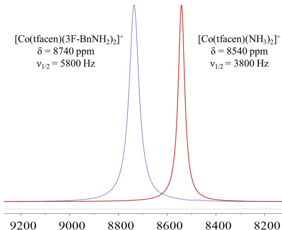
Fig. 2.  $^{59}\text{Co}$  (120 MHz) NMR of spectra of  $[\text{Co}(\text{tfacen})(\text{NH}_3)_2]^+$  (red) and  $[\text{Co}(\text{tfacen})(3\text{F-BnNH}_2)_2]^+$  (blue), obtained in  $\text{D}_2\text{O}$  and  $\text{MeOD-}d_4$ , respectively at 295 K. Chemical shifts are reported relative to  $\text{K}_3[\text{Co}(\text{CN})_6]$  in  $\text{D}_2\text{O}$  at 0 ppm.
