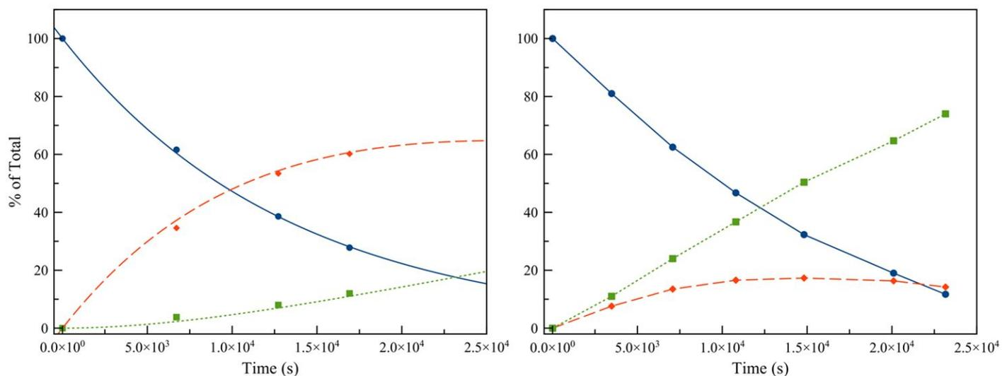
Fig. 6. Representative concentration vs time data for the axial ligand substitution of  $[\text{Co}(3\text{F-salen})(3\text{F-BnNH}_2)_2]^+$  with MeIm at 37 °C in the absence (left) and presence (right) of ascorbate. Concentrations of species (A) (circular markers), (B) (diamond markers), and (C) (square markers) refer to ligand substitution reactants and products shown in Fig. 4.
