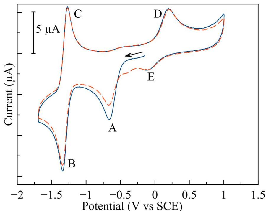
Fig. 3. Cyclic voltammogram of  $[\text{Co}(\text{tfacn})(3\text{F-BnNH}_2)_2]^+$  in DMF with 0.1 M TBAP supporting electrolyte. Potential is referenced to the SCE based on ferrocene ( $E_{1/2}$  0.45 V vs SCE) as internal standard. The first scan is shown as a solid blue line, while the second scan is shown as a dashed, red line.
