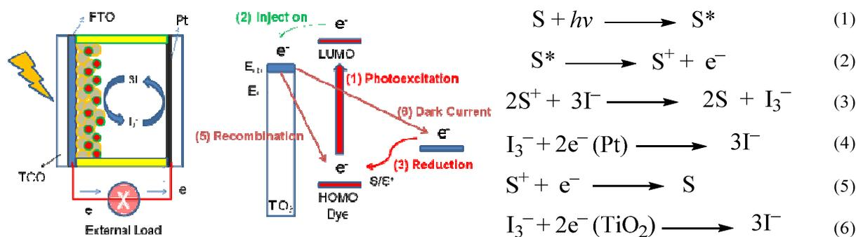
Fig. 1 (a) Schematic design and (b) working principle of a DSSC.
