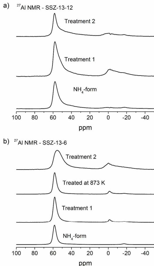
Figure 4. <sup>27</sup>Al MAS NMR of a) SSZ-13-12 samples; NH<sub>4</sub>-form, treated at 773 K and 1073 K, b) SSZ-13-6 samples; NH<sub>4</sub>-form, treated at 773 K, 873 K, and 1073 K.
