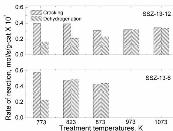
Figure 6. Reaction rates for cracking and dehydrogenation of propane at reaction temperature 773 K over SSZ-13-12 and SSZ-13-6 treated at different pretreatment temperatures.
