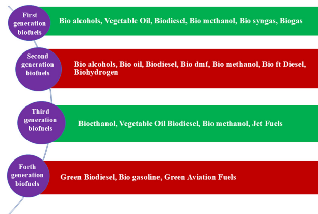
Fig. 2 An in-depth classification of biofuels: advancements from first to fourth generation, exploring feedstock, production technologies, and sustainability aspects.
