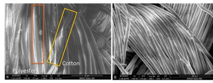
Fig. 27 SEM images to display the structure of the polycotton waste textile prior to acid hydrolysis. The image on the right highlights a significant decrease in cotton fibers, demonstrating the effective selective hydrolysis of the cotton component.<sup>252</sup>
