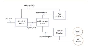
Fig. 22 Block flow diagram of the Shell Oil Company patented process, figure from ref. 221.
