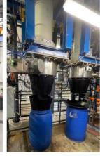
Fig. 19 The Avantium DAWN<sup>™</sup> Pilot plant in Delfzijl, The Netherlands with  $8 \times 230$  l "Fixed bed" reactors for operation in Simulated Moving Bed (SMB) mode (for SMB mode operation, see Fig. S27†).
