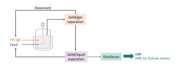
Fig. 24 The biphasic liquid—gas reactor for the continuous production of CMF developed by Origin Materials.<sup>243,244</sup>
