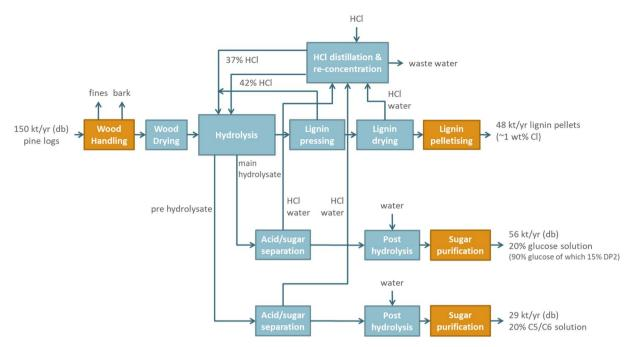
Fig. 20 DAWN Technology™ process block flow diagram: starting from the top-left, the process includes de-barking and drying wood chips, followed by two-stage hydrolysis using different HCl concentrations. The sugar solutions from each hydrolysis stage are collected separately and then post-hydrolyzed to produce monomeric sugars in solution. Lignin is pressed, pelletized, and the sugars are purified before being transported to customers.
