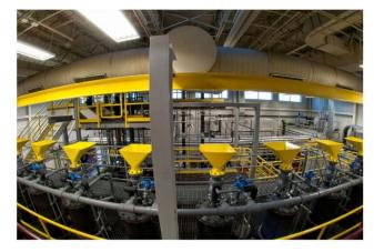
Fig. 18 Top side of the hydrolysis reactors at the Virdia pilot plant in Danville, the yellow conical funnels feed the wood material into the
