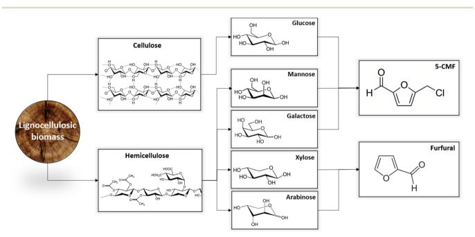
Fig. 25 Lignocellulosic conversion to furanics in an integrated 2-step process developed by Avantium.<sup>239</sup>
