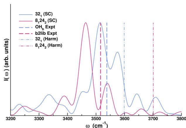
Fig. 2 Semiclassical calculations of the hydrogen-bonded water OH<sub>b</sub> stretch (32<sub>1</sub>, blue) and b2lib combination band (8<sub>1</sub>24<sub>2</sub>, pink) for acetone monohydrate. The zero of energy is set at the ZPE, so that  $I(E)$  is replaced by  $I(\omega)$ .
