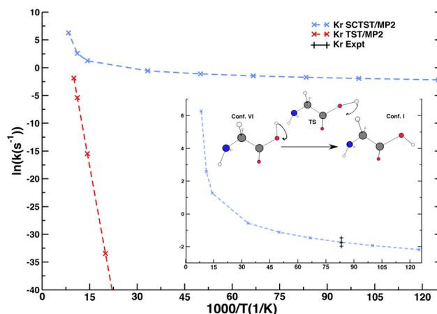
**Fig. 3** Arrhenius plot for glycine interconversion from conformer VI to conformer I in a Krypton matrix. Comparison between classical TST estimate (red), semiclassical SCTST calculation (blue), and experiment (black).
