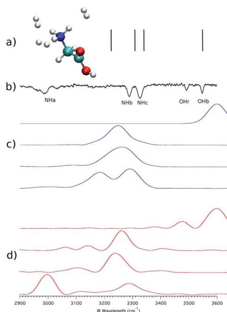
Fig. 1 Vibrational spectra for protonated glycine microsolvated by three  $\text{H}_2$  molecules. Panel (a): harmonic estimates. Panel (b): the experimental spectrum; Panel (c): the quasi-classical trajectory method results; Panel (d): DC-SCIVR calculation. This figure has been reproduced from ref. 47 with permission from the Royal Society of Chemistry, copyright 2018.
