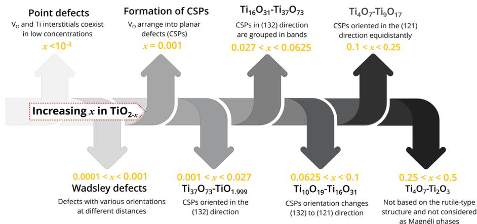
Fig. 3 Formation of different defect induced TiO<sub>2</sub> and phases with increasing  $x$  in TiO<sub>2-x</sub>.
