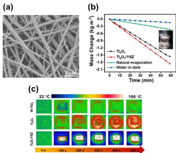
Fig. 21 (a) SEM image of fibrous  $\text{Ti}_4\text{O}_7$  membrane after calcination. (b) Rate of water evaporation from the  $\text{Ti}_4\text{O}_7$  membrane with and without YSZ. (c) Temperatures on the surface of water recorded for  $\text{TiO}_2$ ,  $\text{Ti}_4\text{O}_7$  and  $\text{Ti}_4\text{O}_7/\text{YSZ}$  membranes by an IR thermometer. Reprinted with permission from ref. 229. Copyright 2022, American Chemical Society.
