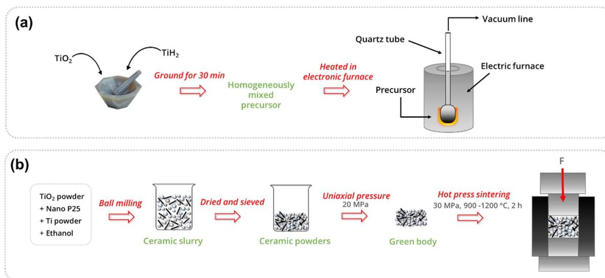
Fig. 11 (a) Schematic representation of the experimental route for the synthesis of titanium suboxides in an electric furnace under vacuum and (b) schematic diagram of the *in situ* hot press sintering technique used to synthesise  $\text{Ti}_4\text{O}_7$ .
