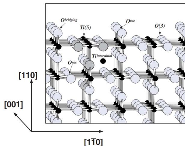
Fig. 2 Ball and stick model of the rutile  $\text{TiO}_2$  (110) surface. Large grey balls represent oxygen atoms and small black balls represent titanium atoms. Two types of point defects that are prevalent in rutile  $\text{TiO}_2$ , oxygen vacancies ( $\text{O}_{\text{vac}}$ ) and Ti interstitials, are shown. Reprinted with permission from ref. 51. Copyright 2003, Springer Nature.
