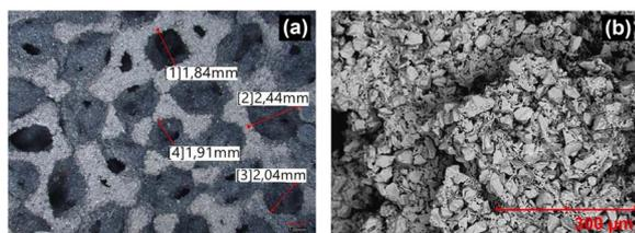
Fig. 23 (a) Porous structure and pore size of 3D printed  $\text{TiO}_x$  electrode and (b) morphology of 3D  $\text{TiO}_x$  as observed from SEM. Reprinted with permission from ref. 240. Copyright 2023, Elsevier.
