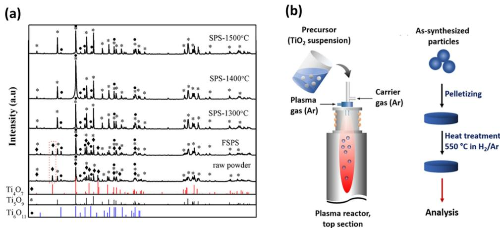
Fig. 13 (a) XRD patterns of raw powder, FSPS sample and samples prepared by conventional SPS at different temperatures.<sup>153</sup> (b) Preparation of  $\text{TiO}_x$  nanoparticles using radiofrequency (RF) induction thermal plasma method (left) and heat treatment of the samples after synthesis to improve their electrical conductivity (right).<sup>13</sup>
