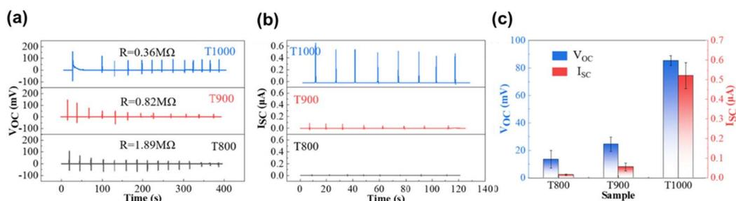
Fig. 22 (a) Measured open circuit voltage ( $V_{\text{OC}}$ ) and (b) short circuit current ( $I_{\text{SC}}$ ) for Magnéli phase nanocrystal films prepared at different temperatures (800–1000 °C) and (c) average peak values of  $V_{\text{OC}}$  and  $I_{\text{SC}}$ . Reprinted with permission from ref. 129. Copyright 2021, American Chemical Society.
