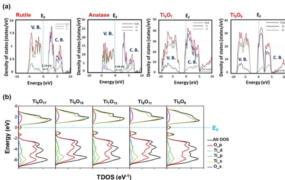
Fig. 9 (a) Normalised DOS diagram for rutile, anatase,  $\text{Ti}_4\text{O}_7$  and  $\text{Ti}_5\text{O}_9$  (ref. 106) and (b) Calculated total DOS of Magnéli phase  $\text{Ti}_n\text{O}_{2n-1}$  ( $5 \leq n \leq 9$ ).<sup>30</sup>
