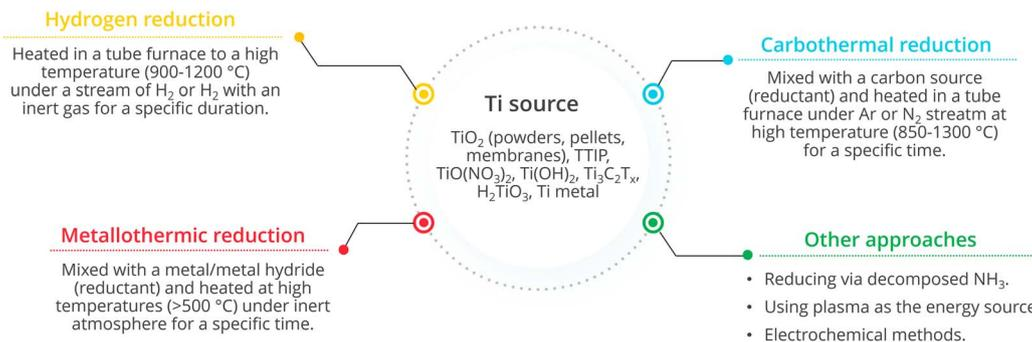
Fig. 10 Different synthesis approaches for Magnéli phase titanium suboxides (TTIP is titanium(IV) isopropoxide and T<sub>x</sub> indicates functional groups) and a typical process for each method.
