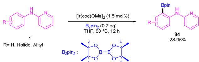
Scheme 49 Ir(III)-catalyzed C–H borylation of 2-anilino-2-pyridines and 2-phenoxy-2-pyridines.
