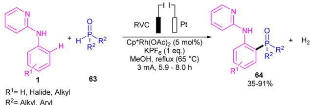
Scheme 37 Rh(III)-catalyzed C–H phosphorylation of *N*-aryl-2-aminopyridines with phosphorous reagents.
