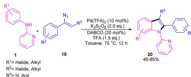
Scheme 10 Pd(II)-catalyzed cyclization of anilines with vinyl azides.
