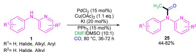
Scheme 16 Pd(II)-catalyzed acylation of *N*-phenyl-2-aminopyridines with DMF and CO.
