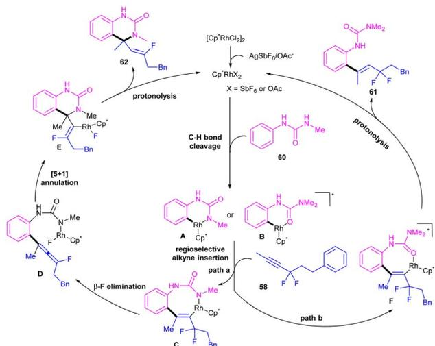
Scheme 36 Plausible mechanism for Rh(III)-catalyzed C–H alkenylation with *N*-pyridylanilines and *gem*-difluoromethylene alkynes.
