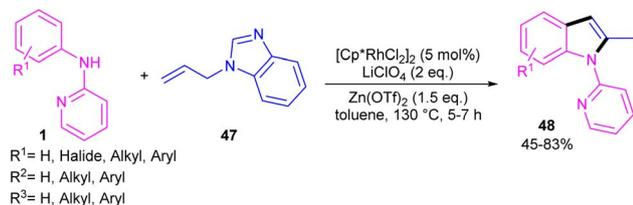
Scheme 28 Rh(III)-catalyzed (3 + 2)-annulation of *N*-phenyl 2-aminopyridine and *N*-allylbenzimidazole.
