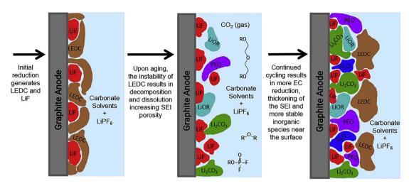
Fig. 2 Schematic diagram of the formation of an SEI film on a graphite anode (reprinted from ref. 37. Copyright 2019, with permission from Elsevier).
