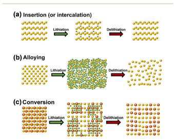
Fig. 1 Schematic diagrams of basic lithium storage principles of the anode materials (a) embedding reaction mechanism, (b) alloying reaction mechanism, (c) transformation reaction mechanism (reprinted from ref. 20. Copyright 2020, with permission from MDPI).
