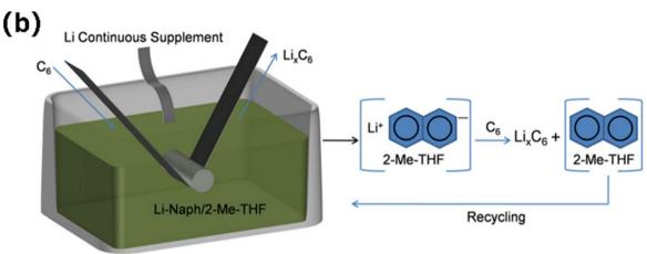
Fig. 15 (a) Geometrical configurations and HOMO energy levels (reprinted from ref. 97. Copyright 2021, with permission from Wiley-VCH). (b) Schematic illustration for the prelithiation reaction of Gr with Naph-Li/2-Me-THF solution (reprinted from ref. 98. Copyright 2022, with permission from Wiley-VCH).
