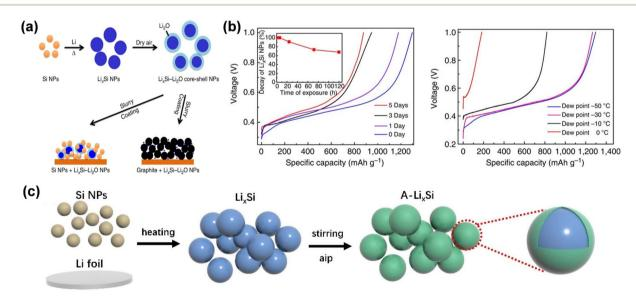
Fig. 9 (a) Schematic diagrams showing Si NPs react with melted Li to form  $\text{Li}_x\text{Si}$  NPs. (b) The capacity retention of  $\text{Li}_x\text{Si}-\text{Li}_2\text{O}$  NPs exposed to dry air with varying durations and air at different humidity levels (reprinted from ref. 69. Copyright 2014, with permission from Springer Nature). (c) Synthesis process for the  $\text{Li}_x\text{Al}_v\text{SiO}_z/\text{Li}_2\text{O}$ -coated  $\text{Li}_x\text{Si}$  (A-Li<sub>x</sub>Si).
