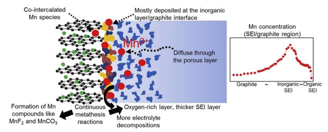
Fig. 5 The spatial distribution of Mn deposited at the SEI/graphite interface (reprinted from ref. 55. Copyright 2015, with permission from Elsevier).
