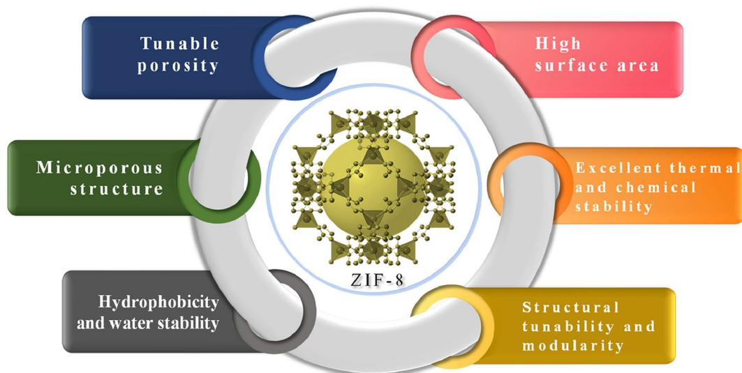
Fig. 2 Schematic representation of various properties of ZIF-8.
