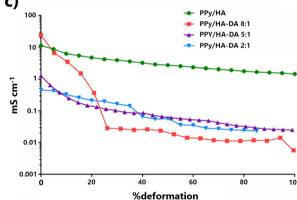
Fig. 13 (a) Conductivities of PPy/HA and PPy/(HA–DA) films on a poly(dimethylsiloxane) substrate. (b) Conductivities of PPy/HA and PPy/(HA–DA) 8:1 films under different humidity conditions. (c) Conductivity as a function of applied stress; conductivity measurements are shown as the mean and standard deviation of n=3. Reproduced, with adaptations, from ref. 233 with permission from Elsevier; copyright © 2017 Elsevier B.V.
