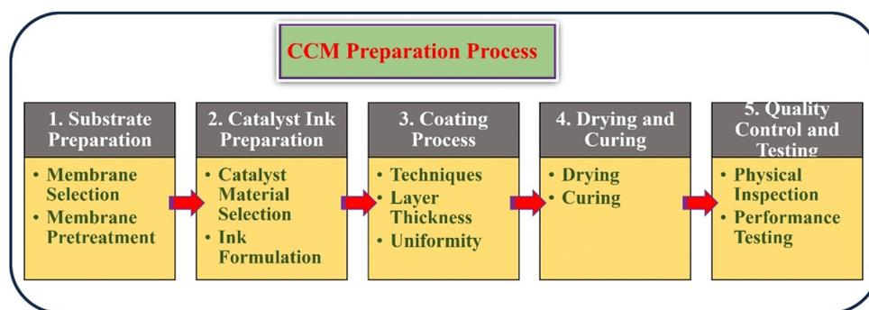
Fig. 3 Schematic sketch of the CCM preparation process.
