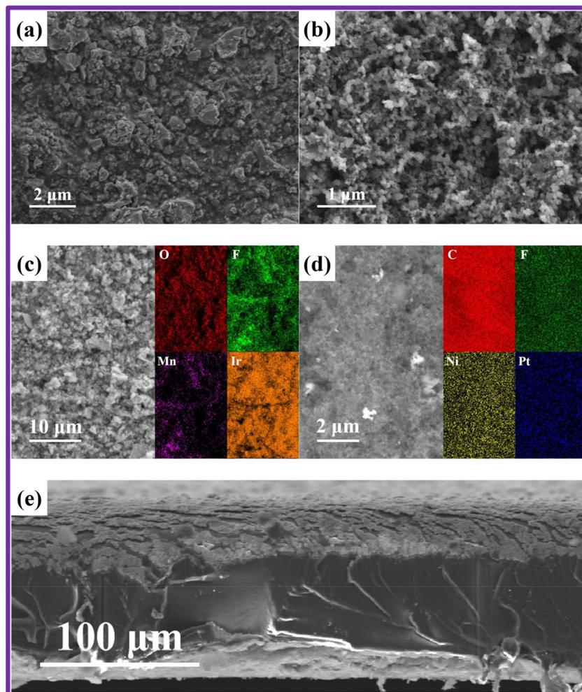
Fig. 4 Microstructural analysis of CCM surface and cross-section. (a) SEM depiction of the anode catalyst layer; (b) SEM portrayal of the cathode catalyst layer; (c) elemental distribution in the anode catalyst layer; (d) elemental distribution in the cathode catalyst layer; (e) SEM visualization of the cross-sectional view. Reproduced with the permission from ref. 77. Copyright 2023, Elsevier.
