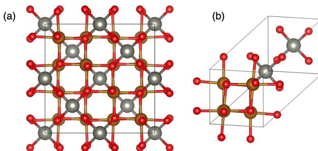
**Figure 1.** Crystal structure of  $MFe_2O_4$  spinels represented by a) the conventional cubic cell and b) the primitive unit cell. Colour scheme: tetrahedral (Td) sites = silver; octahedral (Oh) sites = gold; oxygen = red.
