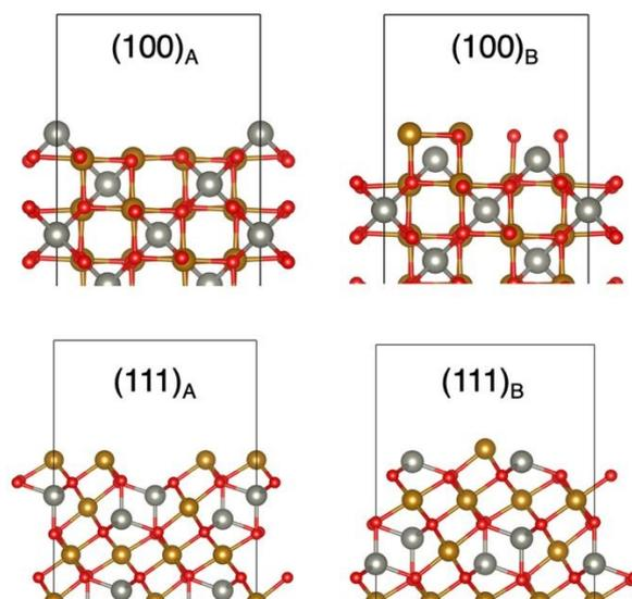
**Figure 2.** Surface structures of  $\text{ZnFe}_2\text{O}_4$  (100) and (111) surface reconstructions leading to stoichiometric and non-polar terminations. Only one side of the slab is shown but the other side of the slab is equivalent by symmetry. Colour scheme: Zn = silver; Fe = gold; oxygen = red.
