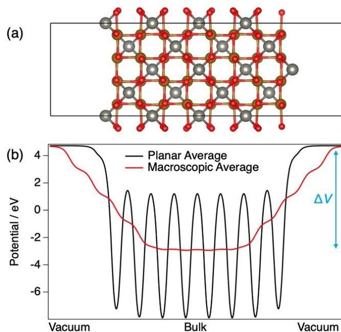
**Figure 6. (a) ZnFe<sub>2</sub>O<sub>4</sub> slab with a (100) termination and (b) the planar-averages of the electrostatic potential.**
