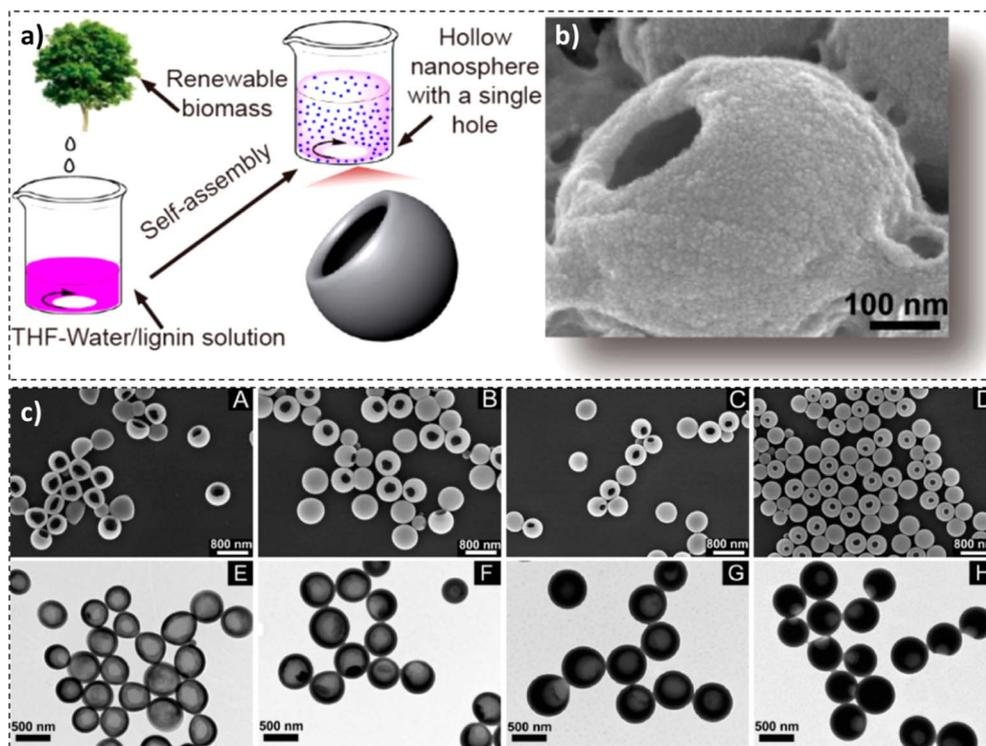
Fig. 5 (a) Synthesis process, (b) SEM image, and (c) SEM images (A–D) and TEM images (E–H) at different predropping lignin concentrations:  $0.5 \text{ mg mL}^{-1}$  (A and E),  $1 \text{ mg mL}^{-1}$  (B and F),  $1.5 \text{ mg mL}^{-1}$  (C and G), and  $2 \text{ mg mL}^{-1}$  (D and H) (reproduced from ref. 107 with permission from ACS, copyright 2017).
