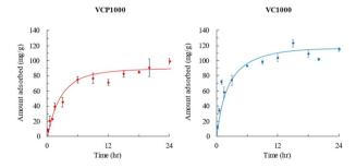
Fig. 5 The effect of contact time on the adsorption of CV onto VCP1000 or VC1000. Initial concentration, 100 mg  $L^{-1}$ ; sample volume, 50 mL; adsorbent, 0.02 g; temperature, 25 °C; contact time, 10 and 30 min and 1, 1.5, 3, 6, 9, 12, 15, 18, 20, and 24 h, 100 rpm.
