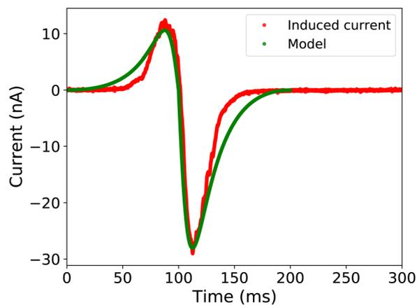
Fig. 6 Induced capacitive current shows qualitative and quantitative agreement with the sliding plate capacitor model. We used  $\sigma_{\text{out}} = -28$   $\mu\text{C m}^{-2}$ ,  $\sigma_{\text{in}} = \sigma_{\text{out}} \exp(-\Delta t/3 \text{ s})$ , and  $v = 0.15$   $\text{m s}^{-1}$  for the simulation.
