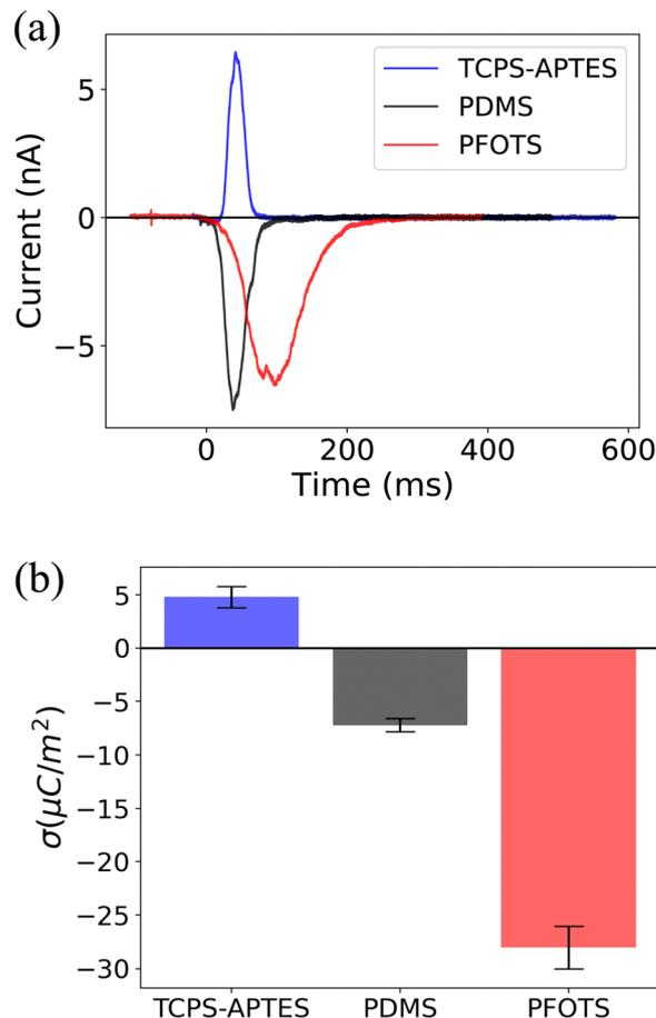
Fig. 3 (a) Capacitive current induced by a grounded sliding drop on glass coated with different hydrophobic surface. (b) Surface charge density ( $\sigma$ ) estimate integrating the current curves in (a). We observe that APTES has a positive surface charge density (positive current peak) whereas glass coated with PDMS and PFOTS has negative surface charge densities (negative peak).
