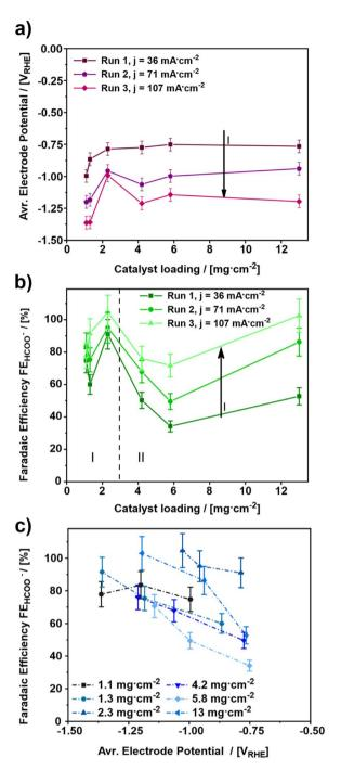
Fig. 1 Influence of the catalyst loading on (a) the average electrode potential for three different applied current densities (36, 71 and 107 mA cm $^{-2}$ ) and (b) the faradaic efficiency for formate after a run time of 11 min each. (c) Shows a combination of the plots a and b. (Measurement conditions: batch reactor, 12 ml electrolyte, 1 M KHCO $_3$ , continuous CO $_2$  supply of 20 ml min $^{-1}$ , start at room temperature, electrolysis time: 45 min each).
