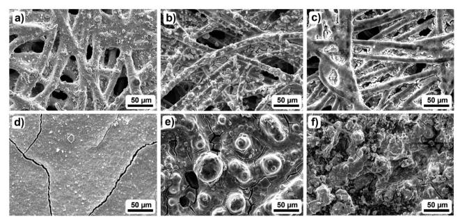
Fig. 4 Exemplary SEM images of the investigated GDEs: (a) and (d) show the pristine GDEs, while (b) and (e) represent the topography after cycle 1. Images (c) and (f) show the GDE after cycle 2 of  $CO_2$  electroreduction to formate for two different catalyst loadings (2.3 mg cm<sup>-2</sup> and 13 mg cm<sup>-2</sup> (top/bottom)). Additional images for the other catalyst loadings are shown in Fig. S7 and S8.†).
