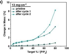
Fig. 6 Vapor sorption measurements of GDEs with different catalyst loadings: (a) 2.3 mg cm<sup>-2</sup> and (b) 13 mg cm<sup>-2</sup>. Vapor adsorption isotherms of the investigated GDEs in different states - pristine, after cycle 1 and after cycle 2. Vapor sorption measurements were conducted at 25 °C with a relative humidity from 0 to 80%; each humidity point was held for 60 min.
