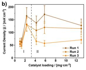
Fig. 2 (a) Exemplary course of the linear sweep voltammograms (LSVs) for the GDE with a catalyst loading of 13 mg cm<sup>-2</sup>. (b) Evaluation of the cathodic current density at  $-1.15\,V_{RHE}$  depending on the catalyst loading. (Measurement conditions: batch reactor, 12 ml electrolyte, 1 M KHCO<sub>3</sub>, continuous CO<sub>2</sub> supply of 20 ml min<sup>-1</sup>, start at room temperature, electrolysis time: 45 min each).
