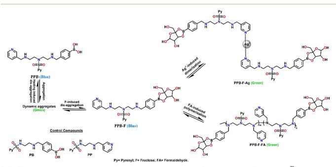
Pictorial representation of the relevant states of the dynamic molecular system 13 in the presence of different analytes.<sup>70</sup>
