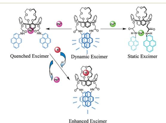
Fig. 12 Pictorial representation of the binding motifs of the probe 26 with  $Cu^{2+}$ ,  $Pb^{2+}$  and  $K^+$  ions (reprinted with permission from ref. 77. Copyright 2006, American Chemical Society).
