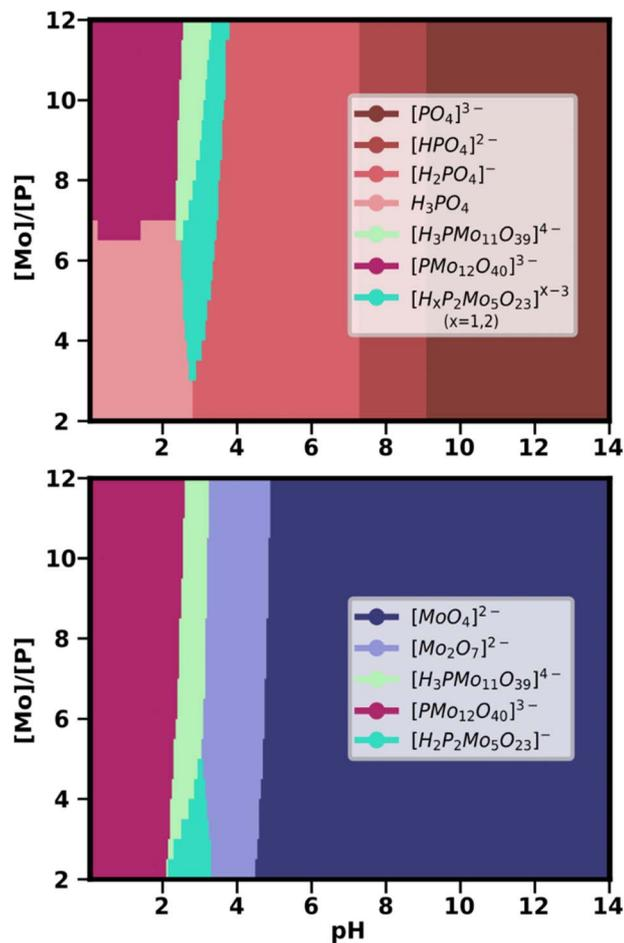
Fig. 5 Speciation phase diagram for the PMo system. The horizontal axis represents pH and the Y axis represents the  $[\text{Mo}]/[\text{P}]$  ratio. The top diagram shows as phosphorus percentage and the bottom one as the molybdenum percentage. The diagrams correspond to two different views of the same speciation phase diagram.
