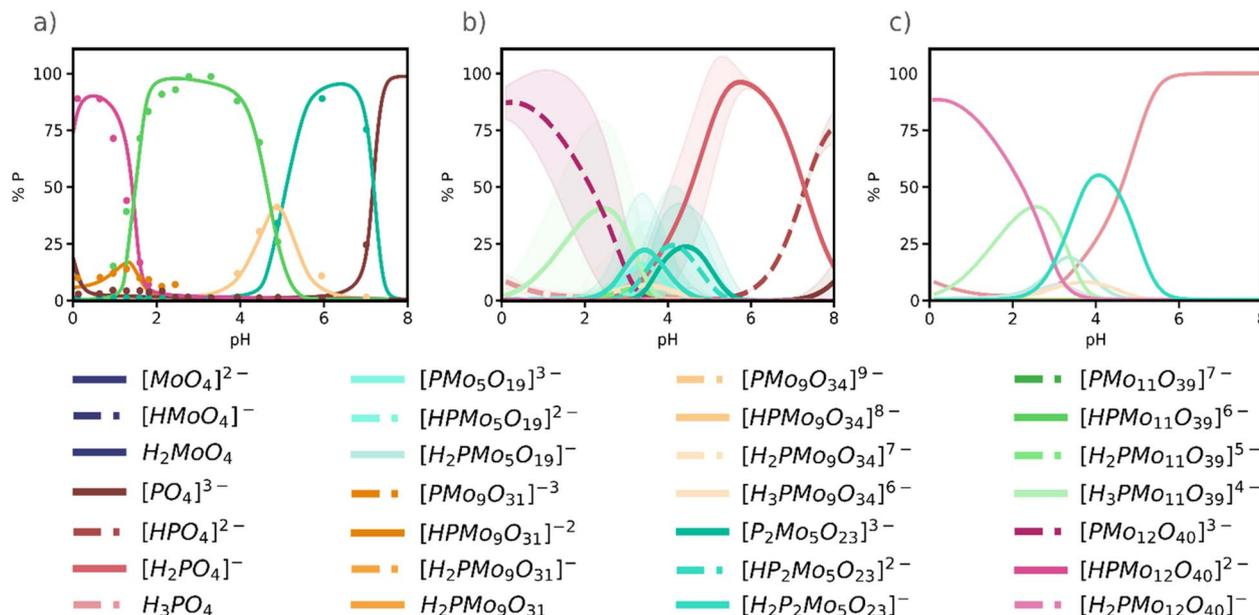
Fig. 4 (a) Experimental speciation diagram for phosphomolybdate system (adapted from Cadot *et al.*<sup>33</sup>); (b) Simulated speciation diagram from 25 761 selected SMs. Lines represent the average value of concentration, and the shading represents the deviation from that value; (c) simulated speciation diagram grouped by nuclearities. For a same nuclearity all protonation states were added into a single line.
