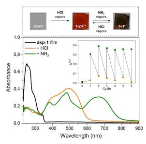
Fig. 9 Top: glass substrate spin-coated with dsp-1 and exposed to ammonia and then hydrochloric acid vapours. Bottom: electronic absorption spectra of the thin film before and after exposure to vapours. Inset: reversibility of pH-switching monitored at 660 nm.
