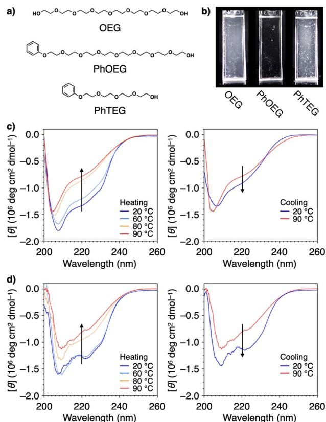
Fig. 9 (a) Molecular structures of OEG, PhOEG, and PhTEG. (b) Photographs of lysozyme in PBS at  $0.037\text{ mM}$  at  $90^\circ\text{C}$  in the presence of (left) OEG, (center) PhOEG, and (right) PhTEG. CD spectral changes of lysozyme in PBS ( $0.037\text{ mM}$ ) in the presence of (c) OEG ( $1.5\text{ mM}$ ) and (d) PhOEG ( $1.6\text{ mM}$ ) in the (left) heating and (right) cooling processes. Arrows indicate the directions of spectral changes.
