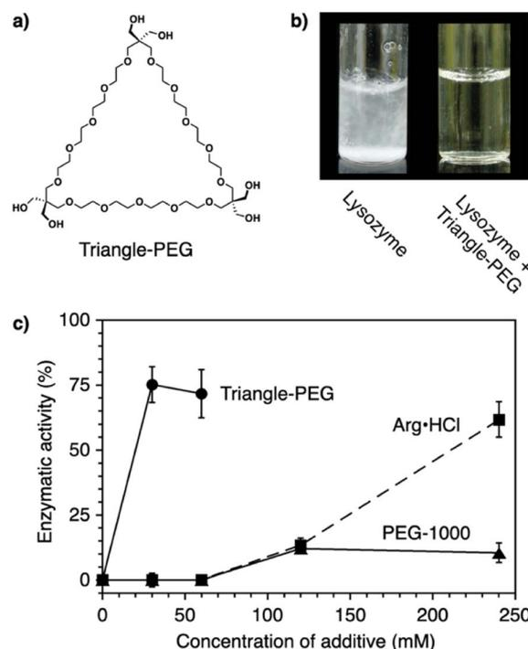
Fig. 8 (a) Molecular structure of triangle-PEG. (b) Photographs of lysozyme in PBS at 3.0 mg mL<sup>-1</sup> (0.21 mM) and 90 °C in the (left) absence and (right) presence of triangle-PEG. (c) Enzymatic activity of lysozyme (3.0 mg mL<sup>-1</sup>) after incubation at 98 °C for 30 min in the presence of triangle-PEG (circles and solid line), PEG-1000 (triangles and solid line), and L-arginine hydrochloride (squares and dashed line).
