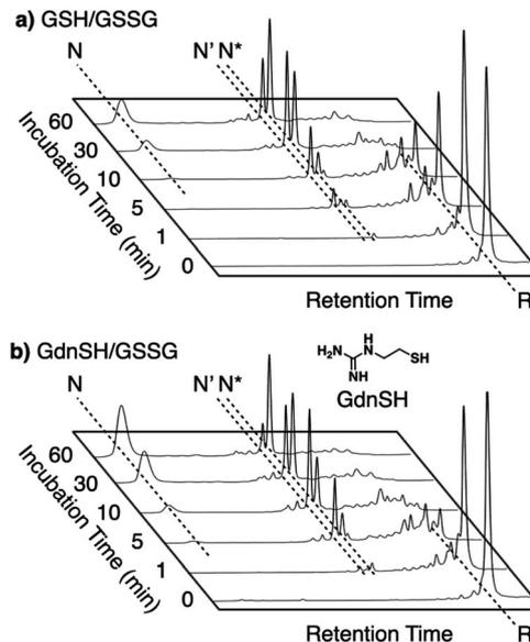
Fig. 11 Time-course reverse-phase HPLC analyses of oxidative folding of BPTI (30  $\mu M$ ) in the presence of GSSG (0.20 mM) and (a) GSH or (b) GdnSH (1.0 mM) using water and  $CH_3CN$  containing 0.05% TFA as eluents with a linear gradient at a flow rate of  $1.0 \text{ mL min}^{-1}$ , with absorption monitored at 229 nm and 25  $^{\circ}C$ .
