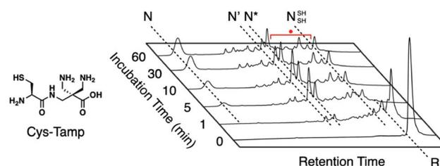
Fig. 13 Time-course reversed-phase HPLC analyses of oxidative folding of BPTI (30  $\mu\text{M}$ ) in the presence of GSSG (0.20 mM) and Cys-Tamp (1.0 mM) using water and  $\text{CH}_3\text{CN}$  containing 0.05% TFA as eluents with a linear gradient at a flow rate of 1.0  $\text{mL min}^{-1}$ , with absorption monitored at 229 nm and 25  $^\circ\text{C}$ .
