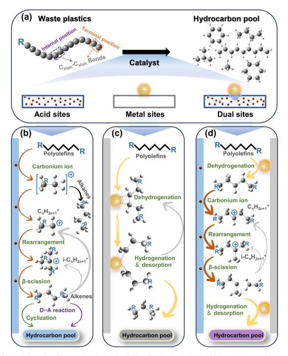
Fig. 2 (a) Schematic illustration of the upcycling of polyolefins via  $C_{aliph}-C_{aliph}$  bond activation. (b-d) Schematic diagrams of the upgradation of polyolefins when  $C_{aliph}-C_{aliph}$  bonds are activated over (b) the acid sites, (c) the metal sites, and (d) the dual sites.
