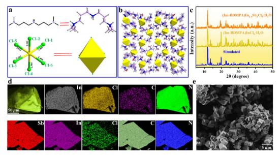
Fig. 1 Structural characterization of (Im-BDMPA)In $_{1-x}$ Sb $_x$ Cl $_6$ ·H $_2$ O: (a) (Im-BDMPA) $^{3+}$  cation and [In/SbCl $_6$ ] $^{3-}$  octahedron; (b) packing structure of the 0D structure viewed along the a-axis; (c) simulated and experimental PXRD patterns; (d) elemental mapping of SEM images; (e) SEM image of a microparticle
