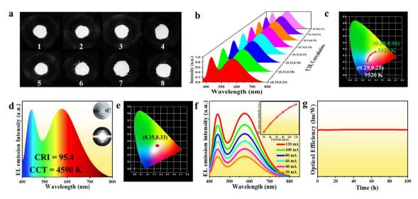
Fig. 4 Characterization of a white LED: (a) photo images of mixed phosphors with varying ratios under 365 nm excitation; (b) PL emission spectra and (c) CIE coordinates of mixed phosphors with varying ratios; (d) EL spectrum of the fabricated white LED (inset: photographs of the fabricated WLED with power off and on); (e) CIE coordinates of the white LED; (f) drive current dependent EL emission spectra; (g) current operating time dependent luminous efficiency.
