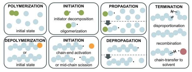
Fig. 8 Reaction steps for radical polymerization (top) and depolymerization (bottom). Initiation requires the generation of radicals from initiator (green) decomposition for the polymerization, and either from a functional end-group activation (orange) or chain scission for the depolymerization. Both have the same termination reactions with recombination, disproportionation, and chain transfer for example to solvent (red).
