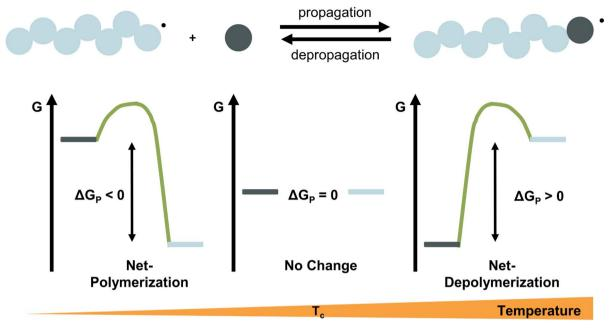
Fig. 1 Schematic representation of the reaction energetics for the propagation-depropagation equilibrium. At low temperature the system favours polymerization, at the ceiling temperature, the system is in equilibrium, and at high temperature depropagation is favoured.
