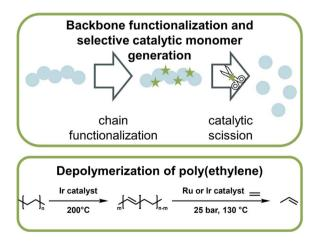
Fig. 16 Schematic overview of catalytic monomer regeneration from previously functionalized polymer backbones with selective catalytic sites (top). Example of depolymerization of dehydrogenated polyethylene with ruthenium and iridium catalysts (bottom) as described in ref. 162.
