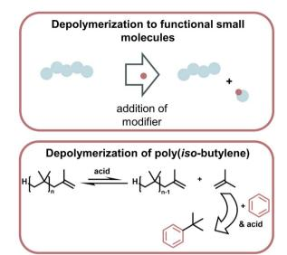
Fig. 15 Schematic overview of depolymerization driven by modification of monomer to make functional small molecules, which then thermodynamically drives the depolymerization (top). Such a system was applied to the depolymerization of poly(iso-butylene) which was driven by the highly enthalpically favoured Friedel-Craft type reaction of the monomer with benzene in the presence of strong acid (bottom) as described in ref. 169.
