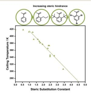
Fig. 4 The effect of phenyl methacrylate's substituents on the ceiling temperature, the larger the substituent the lower the ceiling temperature of the polymerization. Graph reprinted from ref. 90 *Eur. Polym. J.*, 25, 2, B. Yamada, T. Tanaka, T. Otsu, Correlations of ceiling temperature and reactivity with bulkiness of *ortho*-substituent in radical polymerization of phenyl methacrylate, 117–120, Copyright 1989, with permission from Elsevier.
