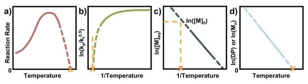
Fig. 7 Four of the most common methods for the ceiling temperature determination from free radical polymerization (a) and (b), and from living polymerization (c) and (d). The orange cross denotes the ceiling temperature, solid lines denote range for which experimental data was acquired, and dashed lines denote extrapolations from the experimental data.
