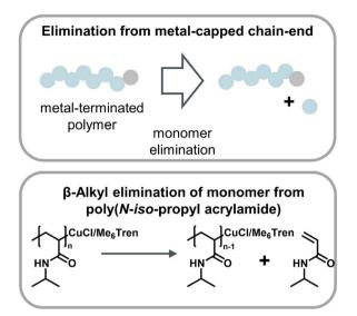
Fig. 14 Scheme of monomer generation from metal-capped polymer chains (top) with the example of poly(N-iso-propyl acrylamide) depolymerization in an aqueous Cu-ATRP system through  $\beta$ -alkyl elimination from copper-terminated chain-ends as described in ref.
