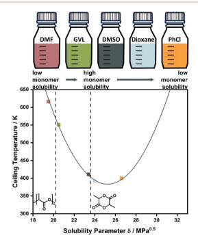
Fig. 5 Changing the ceiling temperature through choice of solvent. The smaller the solubility difference between monomer and solvent, the lower the ceiling temperature. Adapted from ref. 71 "Like recycles like": selective ring-closing depolymerization of poly(L-lactic acid) to Llactide, L. Cederholm, J. Wohlert, P. Olsén, M. Hakkarainen, K. Odelius, Angew. Chem. Int. Ed., 61, 33. Copyright@ 2022 the authors.
