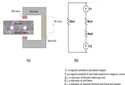
Fig. 5 (a) Electromagnetic corrosion detection device schematic diagram, (b) equivalent model for the electromagnetic set-up.<sup>34,35</sup>
