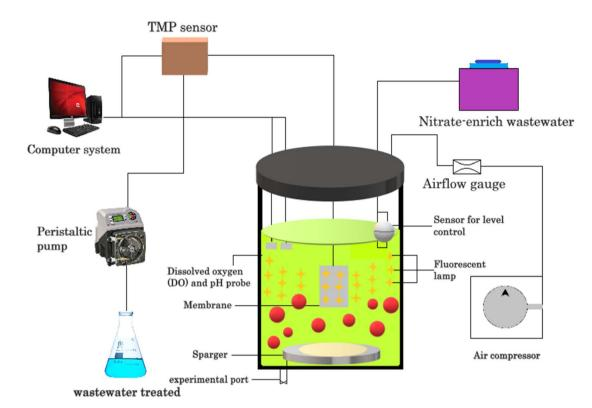
Fig. 6 Pollutant removal through algae membrane reactors.
