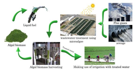
Fig. 1 Typical algae-based wastewater treatment.
