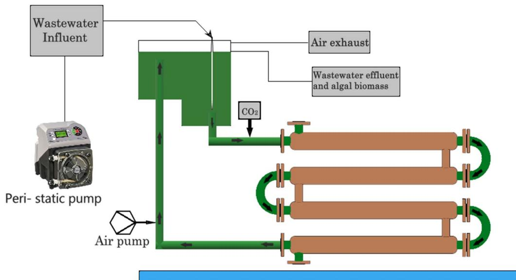
Fig. 7 Lab-scale closed photobioreactor for pollutant removal.
