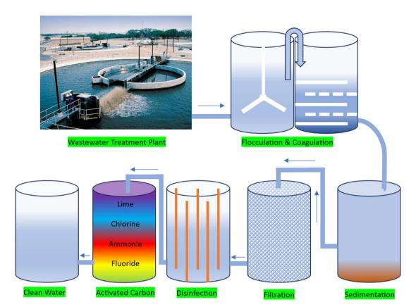
Fig. 4 Stages in wastewater treatment plant.
