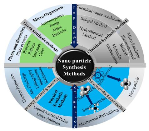
Fig. 5 Overview of nanoparticles synthesis methods: top-down and bottom-up approaches.
