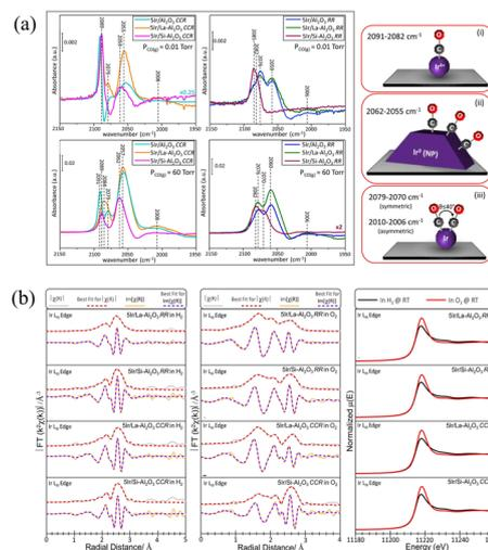
Fig. 7 (a) *In situ* FTIR spectra and CO vibrational features for the catalysts upon CO adsorption. (b) *In situ* XAFS data of the catalysts. Reprinted with permission from ref. 87. Copyright 2022 Elsevier.
