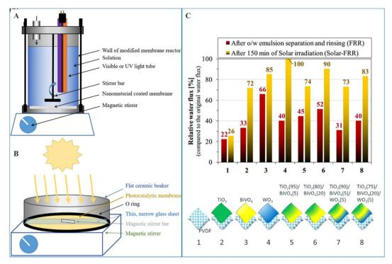
Fig. 8 Schematic figure of (A) the photoreactor used for the comparison of photocatalytic activities of different  $TiO_2/WO_3$  nanocomposite-covered membranes and (B) the experimental setup used for the solar photocatalytic membrane cleaning experiments, (C) solar photocatalytic flux recoveries after 150 min of solar irradiation of the contaminated membranes (coating compositions are defined under the graph. The numbers in the brackets represent percent composition of the nanocomposites).
