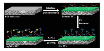
Fig. 5 Schematic illustration of the fabrication of AgNC-modified thin-film composite (AgNC-TFC) membrane (reproduced from ref. 50 with permission from American Chemical Society).
