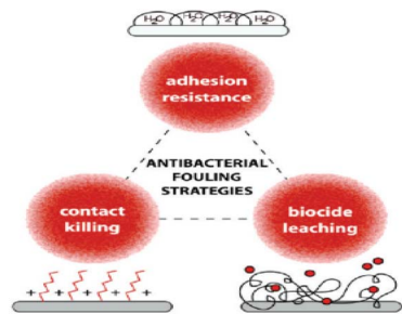
Fig. 15 Polymer-based thin film antimicrobial mechanisms (reproduced from ref. 143 with permission from American Chemical Society).
