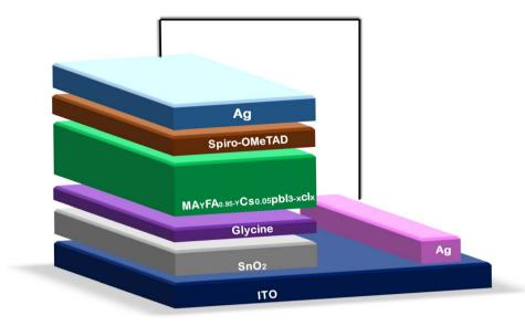
Fig. 7 Schematic of the device architecture of an SnO<sub>2</sub>-based PSC.
