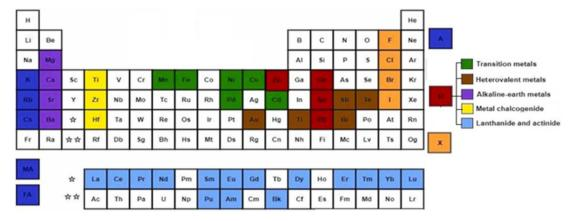
Fig. 3 Elements used in perovskite ABX<sub>3</sub>.
