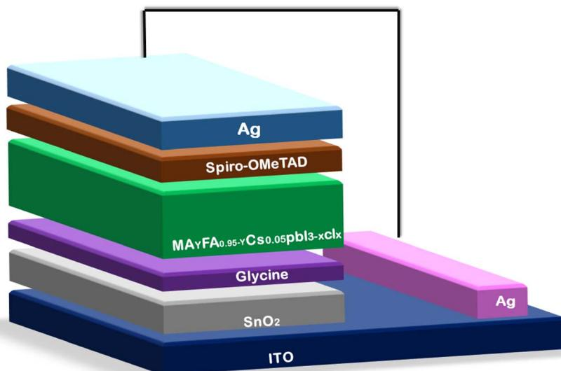
Fig. 7 Schematic of the device architecture of an SnO<sub>2</sub>-based PSC.
