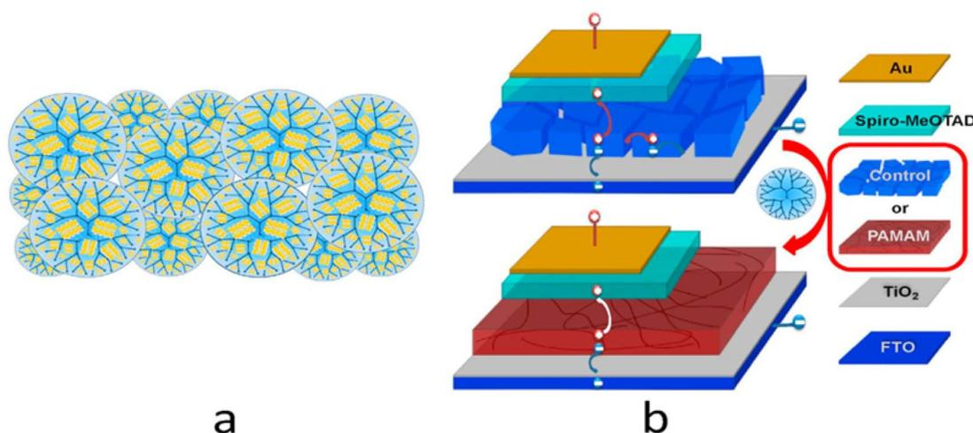
Fig. 13 (a) Schematic depiction of perovskite morphology regulation by PAMAM dendrimers. (b) Device structure of unmodified and PAMAM-modified perovskite photovoltaic devices.<sup>176</sup>
