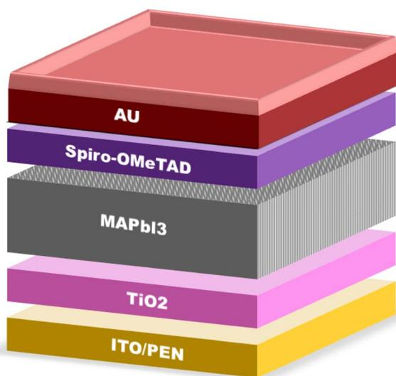
Fig. 5 Architecture of c-TiO<sub>2</sub>-based PSCs.
