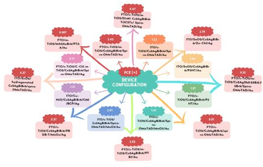
Fig. 15 Device architecture and photovoltaic parameters of HDP-based solar cells.
