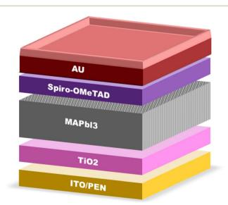
Fig. 5 Architecture of c-TiO<sub>2</sub>-based PSCs.
