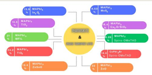
Fig. 6 Effect of different CTLs on the performance of PSCs.
