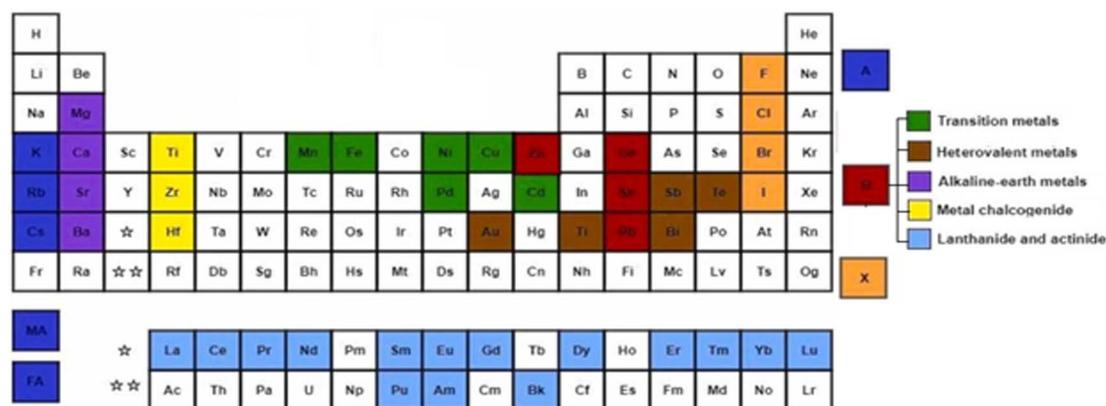
Fig. 3 Elements used in perovskite  $ABX_3$ .
