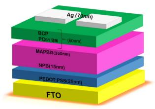
Fig. 14 Structure of the PSC based on NPB
