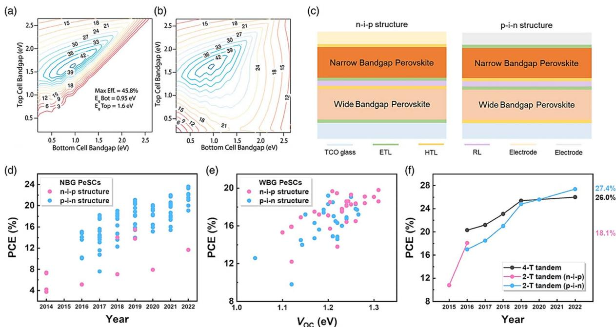
Fig. 16 (a) Maximum efficiency limits for a 2-T tandem solar cell and (b) panel. (c) Configuration of a 2-T PTSC. (d) Efficiency of narrow bandgap (NBG) Sn–Pb PSCs with a bandgap range of 1.17–1.3 eV. (e) Efficiency and  $V_{OC}$  graph of large bandgap (WBG) Pb-based PSCs with a bandgap range of 1.7–1.8 eV. (f) PCE for 2-T and 4-T PTSCs over time. (a and b) Ref. 212.
