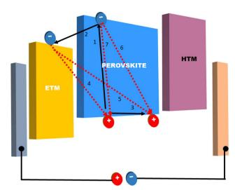
Fig. 4 Energy levels with charge transfer processes inside a PSC.
