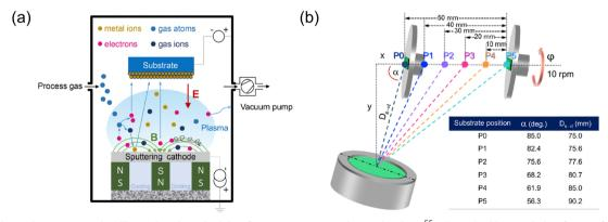
Fig. 3 (a) Schematic representation illustrating the principle of magnetron sputtering technology,<sup>55</sup> adapted with permission from ref. 55, copyright 2020 by Elsevier Ltd and Techna Group S.r.l. (b) Diagram of the magnetron sputtering with glancing angle deposition (MS-GLAD) technique,<sup>56</sup> indicating that the substrate can be adjusted from positions P0 to P5, adapted with permission from ref. 56, copyright 2021 by Elsevier Ltd and Techna Group S.r.l.
