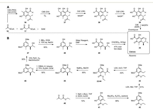
Scheme 3 Citrinin 35 syntheses. (A) Biosynthetic pathway; (B) chemical synthesis pathway. OX: oxygenase/oxidase, OR: oxidoreductase, SDR: short-chain dehydrogenase/reductase. DIBAL-H: diisobutylhydroaluminum, TFA: trifluoroacetic acid.
