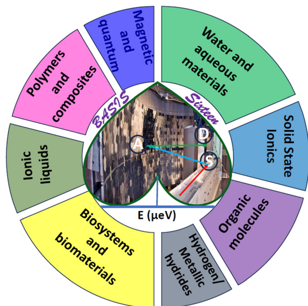
Fig. 1 Overview of the different types of materials studied using BASIS. Also included is the direction of an incident neutron (red arrow) hitting the sample (S), which, after scattering (blue arrow) from the sample, gets backscattered (green arrow) from the Silicon analyzer panel (A) to the detectors (D), resulting in a quasielastic spectrum as a function of energy transfer (the dark-green peak at the base of the heart).
