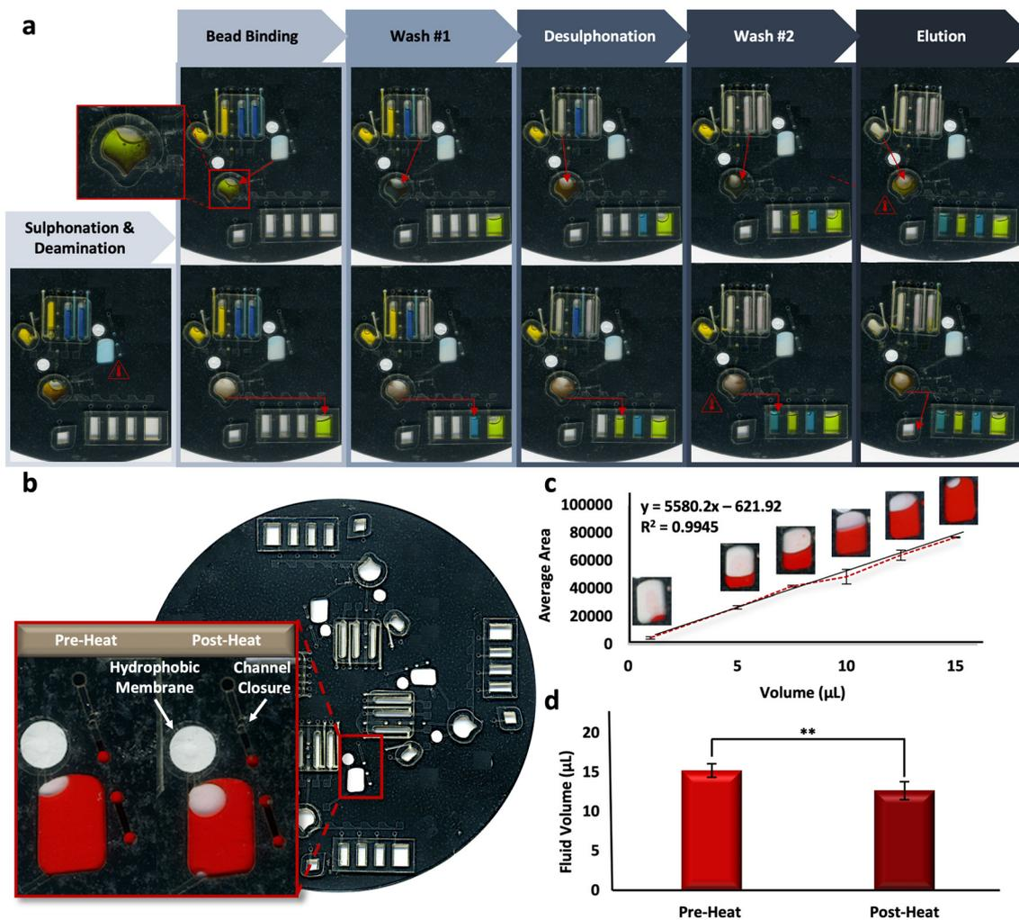
**Fig. 4** Fluidic dye studies. **a**, Digital scans showing one representative dye study. **b**, Digital scans of the bisulfite conversion chamber pre- and post-heating associated with the initial incubation steps (e.g., denaturation, followed by sulphonation and deamination). **c**, Calibration curve corresponding to the average pixel areas of digital scans of bisulfite conversion chambers loaded with Allura red dye. **d**, Quantification of fluid loss pre- and post-heating protocol.
