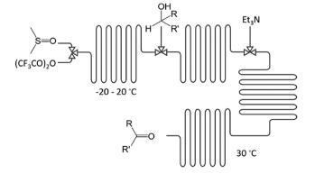
Fig. 3 Flow chemistry applied to sequential multi-step Swern-Moffatttype oxidation.
