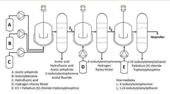
Fig. 20 BHC's 3-step ibuprofen production process.
