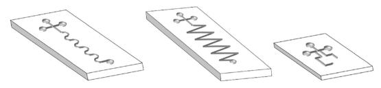
Fig. 16 Micromixer designs used for wastewater treatment.
