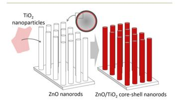
Fig. 8  $\,^{7}$  TiO $_{2}$  nanoparticle-coated ZnO nanorod arrays grown in the capillaries of a photocatalytic microreactor.
