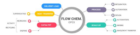
Fig. 9 Flow chemistry OPEX costs sorted by relevant engineering and process viewpoints.
