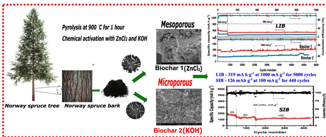
Fig. 2 Synthesis of carbon anodes prepared using different chemical activation with  $\text{ZnCl}_2$  (Biochar-1) and  $\text{KOH}$  (Biochar-2) and tested in LIBs and SIBs. Reproduced with permission.<sup>41</sup> Copyright 2022, American Chemical Society.
