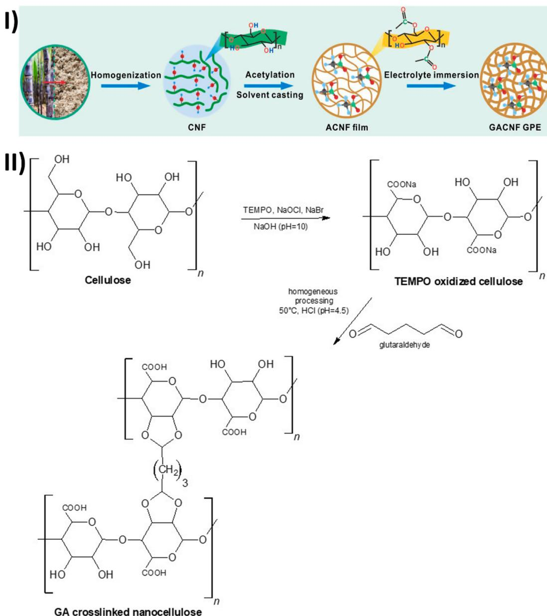
Fig. 6 (I) A scheme of preparation of acetylated cellulose nanofibril-based gel polymer electrolyte (GPE). Reproduced with permission.<sup>109</sup> Copyright 2022, Elsevier. (II) Scheme for preparation of glutaraldehyde crosslinked nano cellulose-based gel polymer electrolyte (GPE).
