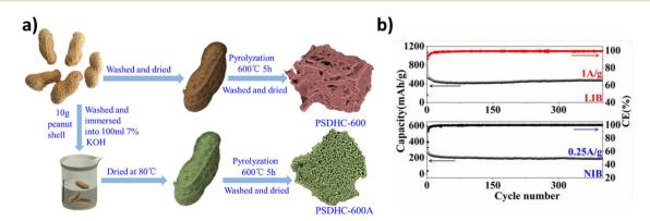
Fig. 3 (a) Synthesis routes for the preparation of hard carbons PSDHC-600 and PSDHC-600A. (b) Cycling performances of peanut shell-derived hard carbon for LIBs and SIBs. Reproduced with permission.<sup>52</sup> Copyright 2015, Elsevier.
