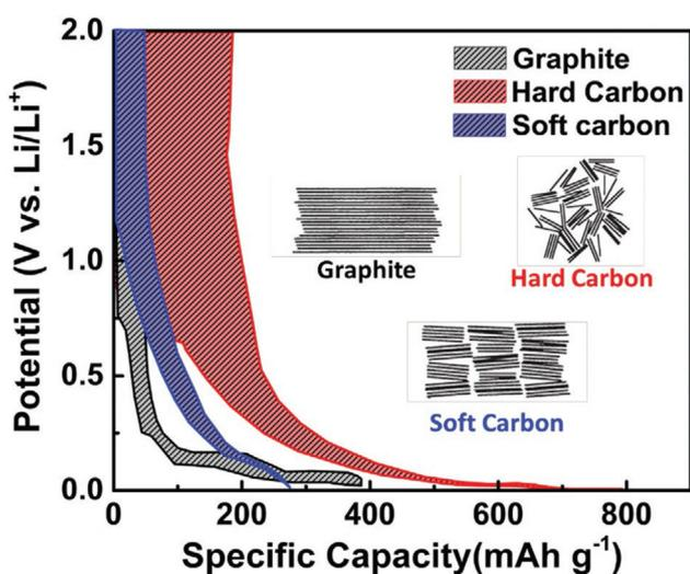
Fig. 1 Voltage profiles comparison between Gr, hard carbon, and soft carbon. Reproduced with permission.<sup>45</sup> Copyright 2001, Wiley-VCH GmbH.
