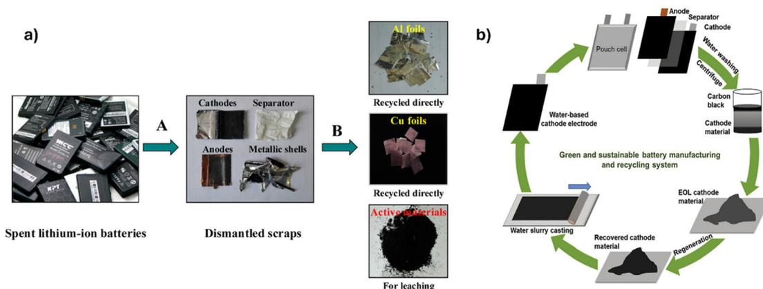
**Fig. 10** (a) The spent LIBs were dismantled from the leaching experiments and recycled secondary materials *via* direct recycling. Reproduced with permission.<sup>179</sup> Copyright 2015, American Chemical Society. (b) A sustainable manufacturing approach for the NMC-based cathodes from the spent LIB. Reproduced with permission.<sup>149</sup> Copyright 2020, Elsevier.
