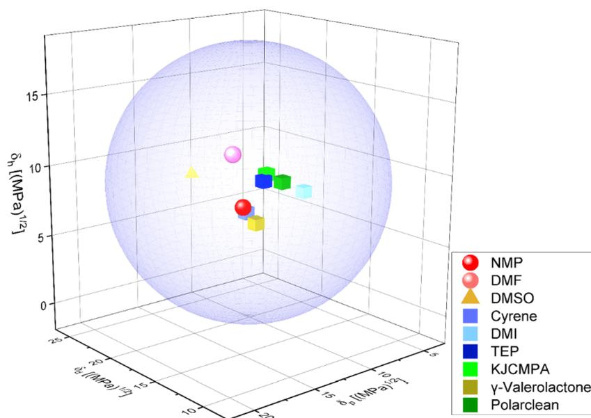
**Fig. 8** Hansen sphere indicating solvents compatible with PVDF binder. Toxic and prohibited solvents (NMP and DMF) are marked with small spheres, less preferable solvent (DMSO) with a triangle, and preferred sustainable solvents (Cyrene, DMI, TEP, KJCMPA,  $\gamma$ -valerolactone, and Polarclean) with cubes.
