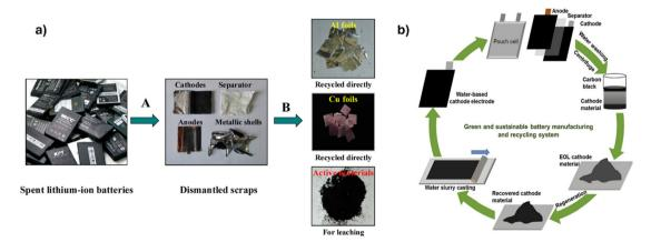
Fig. 10 (a) The spent LIBs were dismantled from the leaching experiments and recycled secondary materials via direct recycling. Reproduced with permission.<sup>179</sup> Copyright 2015, American Chemical Society. (b) A sustainable manufacturing approach for the NMC-based cathodes from the spend LIB. Reproduced with permission. 149 Copyright 2020, Elsevier.
