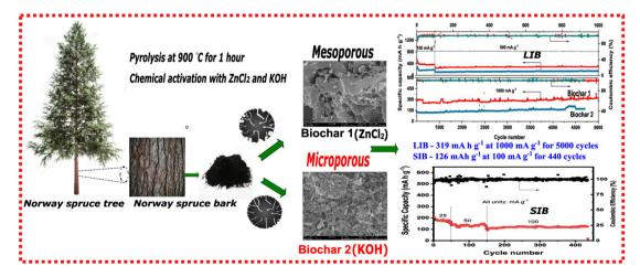
Fig. 2 Synthesis of carbon anodes prepared using different chemical activation with ZnCl<sub>2</sub> (Biochar-1) and KOH (Biochar-2) and tested in LIBs and SIBs. Reproduced with permission.<sup>41</sup> Copyright 2022, American Chemical Society.
