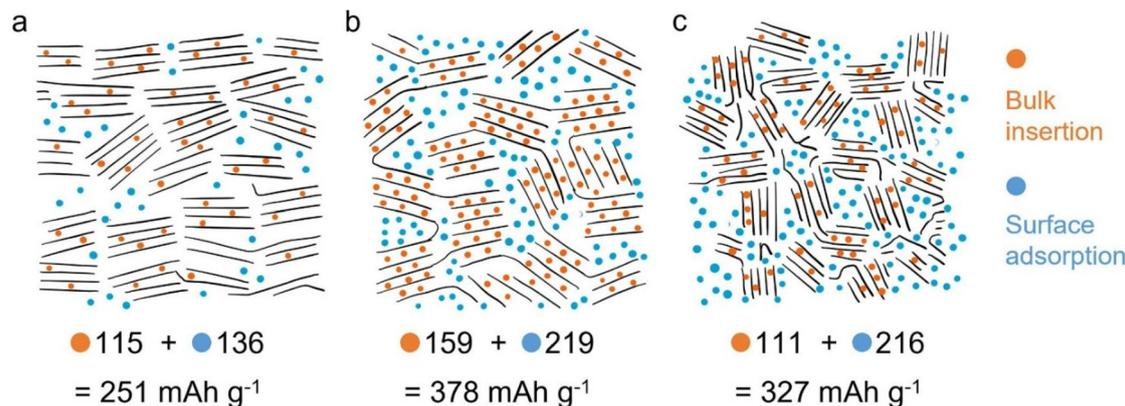
Fig. 5 Proposed K-ion storage mechanisms in L700 (a), M700 (b), and H700 (c). Reproduced with permission.<sup>79</sup> Copyright 2022, Elsevier.
