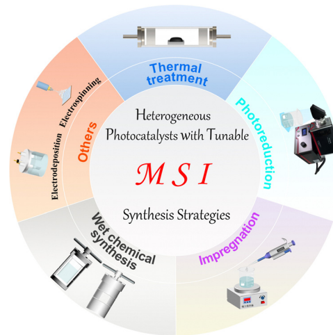
Fig. 2 Summary diagram of the typical preparation methods for heterogeneous photocatalysts with MSIs.
