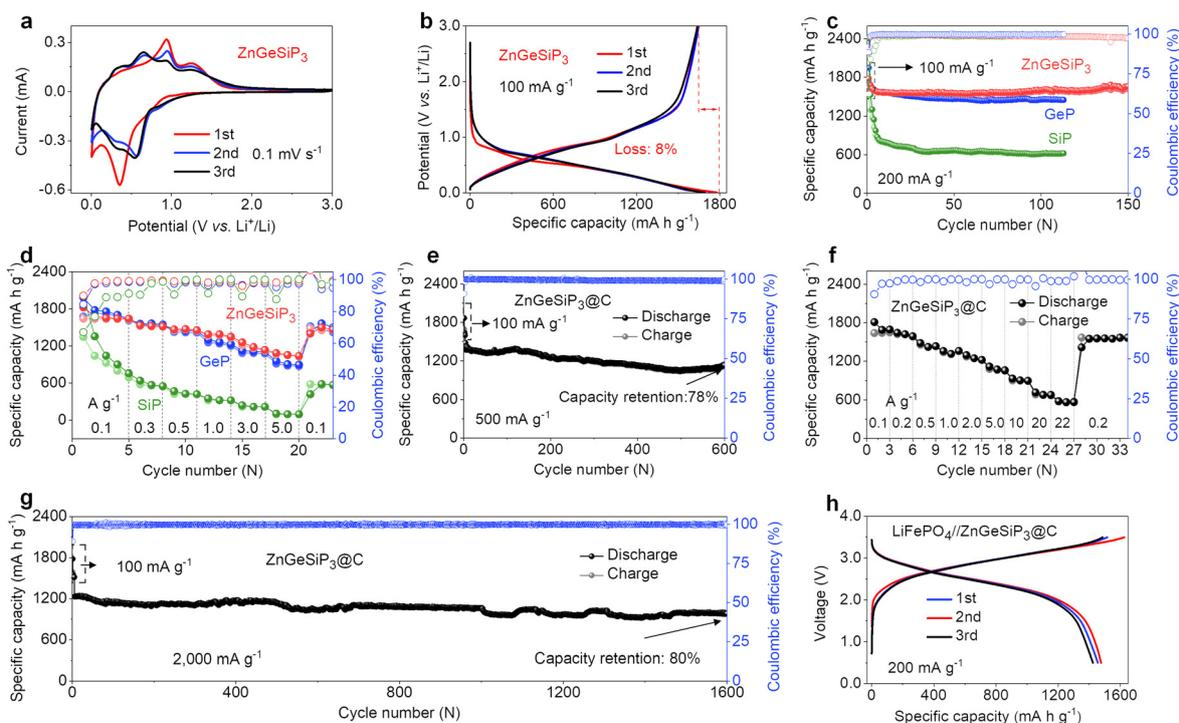
Fig. 2 Electrochemical Li-storage properties of ZnGeSiP<sub>3</sub>, GeP, and SiP. (a) Cyclic voltammetry. (b) GCD profiles. (c) Cycling stability. (d) Rate performance. (e) Cycling stability at 500 mA g<sup>-1</sup>. (f) Rate performance. (g) Cycling performance at 2000 mA g<sup>-1</sup>. (h) GCD profiles of the LiFePO<sub>4</sub>/ZnGeSiP<sub>3</sub>@carbon full cell.
