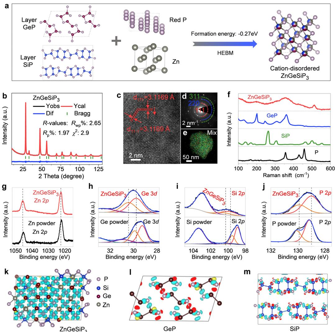
Fig. 1 Synthesis, characterization and disordered lattice analysis of  $\text{ZnGeSiP}_3$ . (a) Synthetic scheme. (b) XRD refinement. (c) HRTEM and (d) SAED. (e) Elemental mappings. (f) Raman spectra. (g)–(j) XPS analysis. (k)–(m) Charge density difference.
