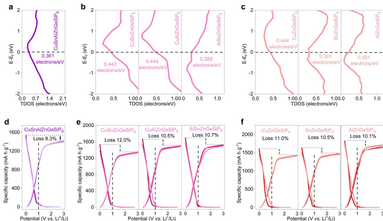
Fig. 6 TDOS calculations and GCD profiles of multiple mixed-cation GeP-based compounds of CuSnAlZnGeSiP<sub>6</sub>, CuSn(or Al)ZnGeSiP<sub>5</sub>, SnAlZnGeSiP<sub>5</sub>, and Cu(or Sn, or Al)ZnGeSiP<sub>4</sub>. (a)–(c) Total density of states (TDOS) profiles. (d)–(f) Initial three charge and discharge profiles.
