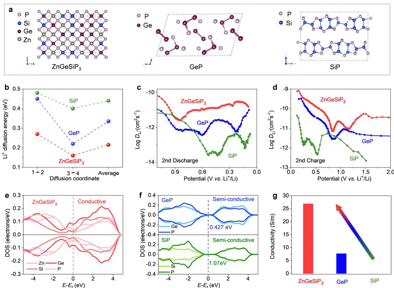
Fig. 4 Charge transport properties of ZnGeSiP<sub>3</sub>, GeP, and SiP. (a) Supercells used for first-principles calculations. (b) Li-ionic hopping energy barriers. (c) and (d) Li-ionic diffusion coefficients derived from GITT measurements. (e) and (f) Projected density of states (PDOS) profiles. (g) Electronic conductivity.
