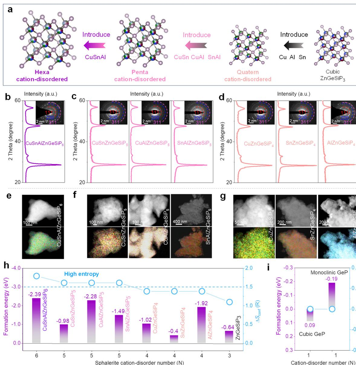
Fig. 5 Characterization and calculations of multiple disordered-cation GeP-based compounds of  $\text{CuSnAlZnGeSiP}_6$ ,  $\text{CuSn}(\text{or Al})\text{ZnGeSiP}_5$ ,  $\text{SnAlZnGeSiP}_5$ , and  $\text{Cu}(\text{or Sn, or Al})\text{ZnGeSiP}_4$ . (a) Schematic of cationic regulation. (b)–(d) XRD and SAED images. (e)–(g) EDS mappings. (h) and (i) Formation energies along with the configurational entropy.
