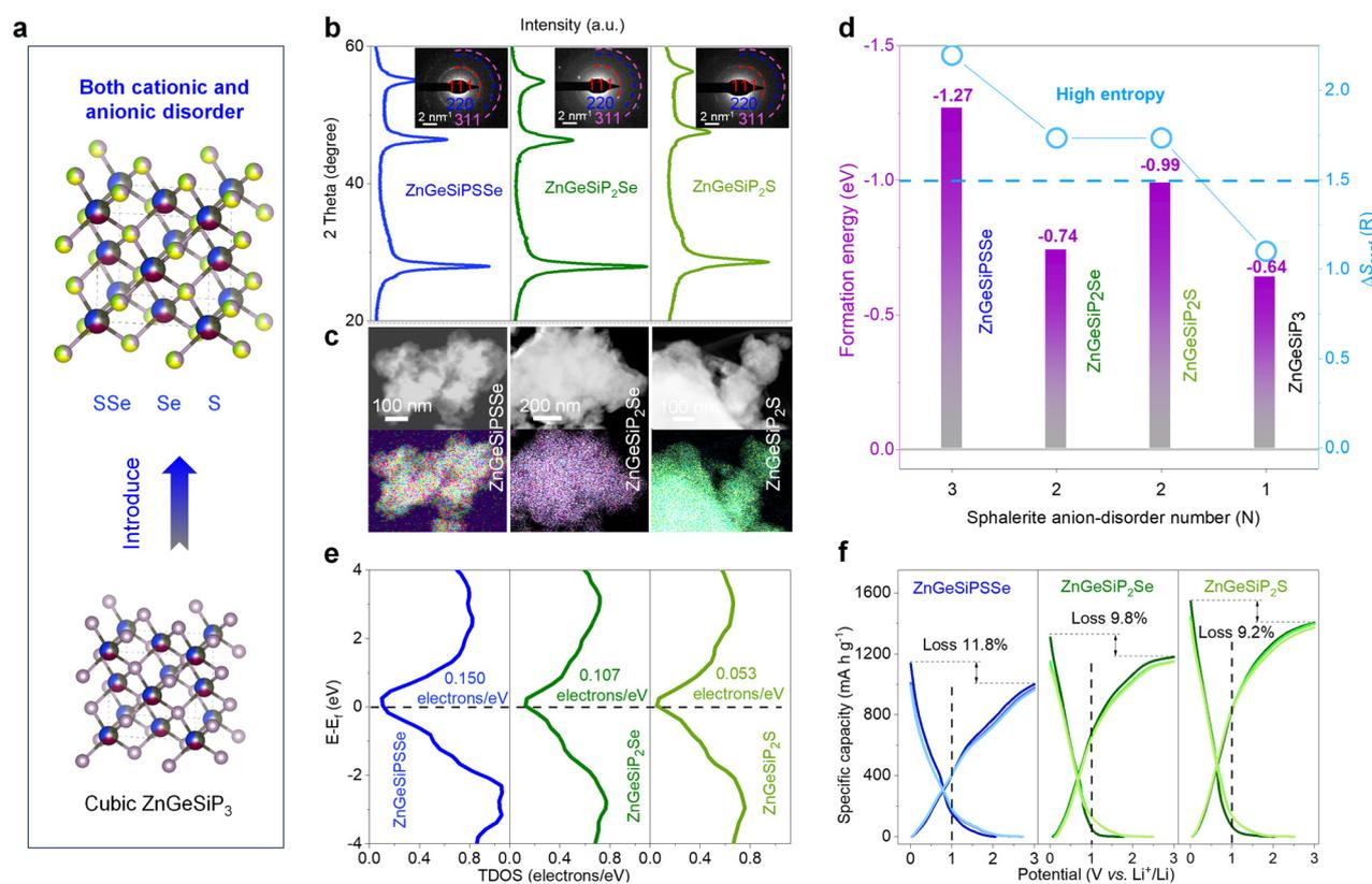
Fig. 7 Characterization, calculations and Li-storage performances of high entropy both disordered-cation and -anion compounds ZnGeSiPSSe and ZnGeSiP<sub>2</sub>Se(or S). (a) Scheme of anionic regulation. (b) XRD and SAED patterns. (c) EDS mappings. (d) Formation energy coupled with the configurational entropy. (e) TDOS profiles. (f) First three charge and discharge profiles.
