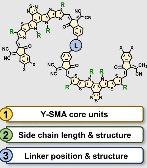
Fig. 8 General design considerations for Y-based DSMA.
