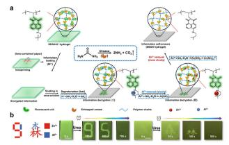
(a) Schematic illustration of urease-containing fluorescent hydrogel for instantaneous multi-level fluorescence information storage. (b) Encryption-decryption-self-erasing process of encoded information during the urease-urea catalyzed reaction.<sup>55</sup> Reprinted with permission from ref. 55 (Copyright 2021 John Wiley and Sons).
