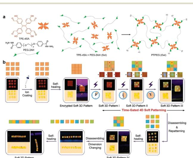
Fig. 17 (a) Diagrammatic representation of the PTPEG gel preparation process. (b) The photos of time-gated 4D soft pattern generated from PTPEG gel coating with ions.<sup>94</sup> Reprinted with permission from ref. 94 (Copyright 2021 John Wiley and Sons).
