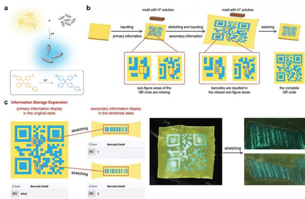
Fig. 14 (a) Interactions between  $(\text{Me}_2\text{N})_2\text{-TPE-Py}$  and LAPONITE<sup>®</sup> XLS under acid stimulation. (b) The encoding process of multiple information, including a QR code and two barcodes. (c) The decryption of hidden QR code and barcodes under UV irradiation and mechanical stretching.<sup>93</sup> Reprinted with permission from ref. 93 (Copyright 2022 John Wiley and Sons).
