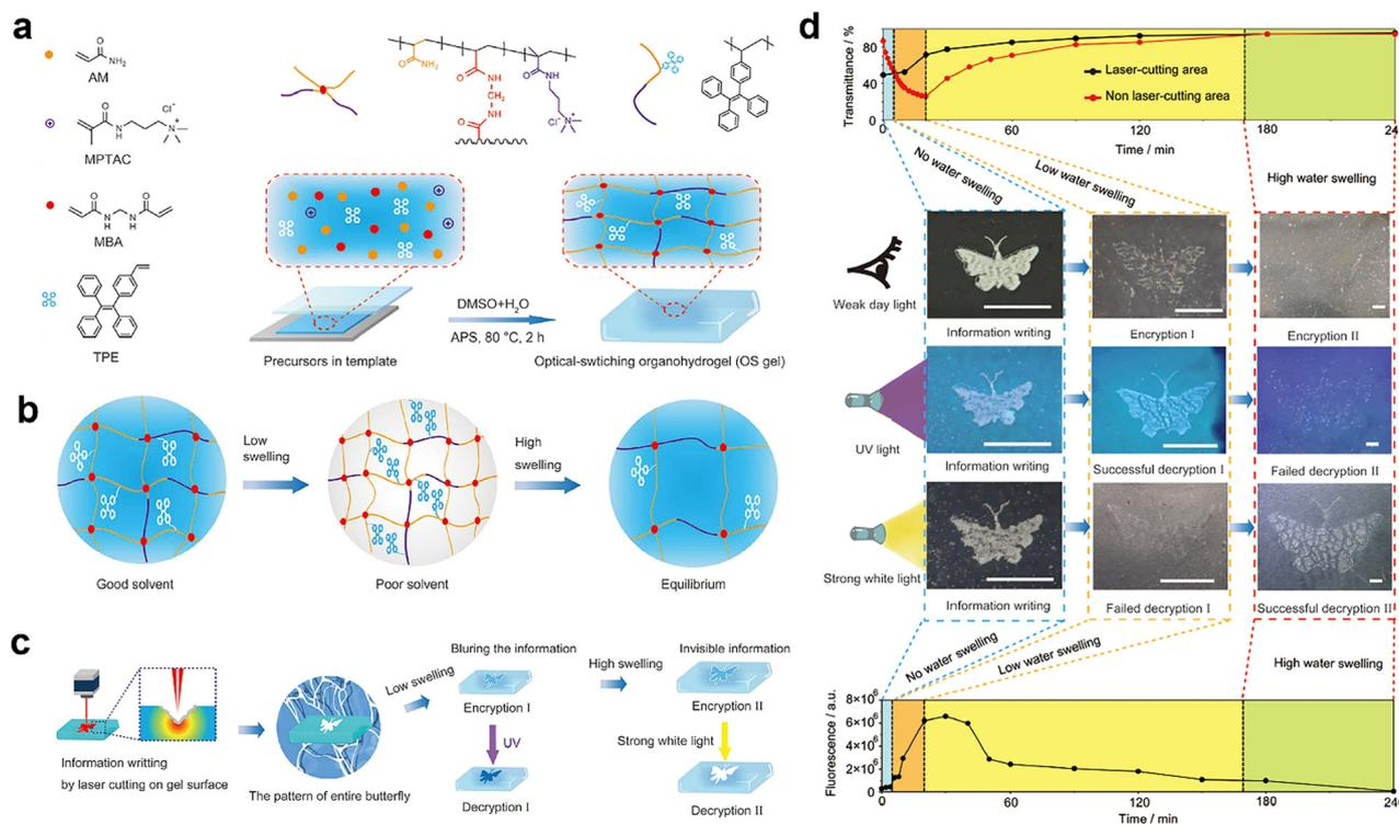
Fig. 3 (a) Design and fabrication of an optical-switching organohydrogel (OS gel). (b) Swelling properties of the OS gel in different conditions. (c) Information encoding and its encryption–decryption process carried out on the surface of the OS gel. (d) Multistage information encryption and decryption based on swelling performance.<sup>66</sup> Reprinted with permission from ref. 66 (Copyright 2022 John Wiley and Sons).
