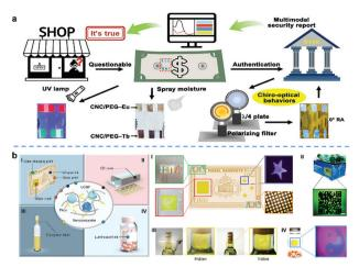
Fig. 20 SRP-based information-storage materials for monetary and product security. (a) CNC-derived photonic composite labels used for banknote anti-counterfeiting.<sup>68</sup> (b) Anti-counterfeiting labels based on PAzo/ UCNP nanocomposites.<sup>99</sup> Reprinted with permission from ref. 68 (Copyright 2022 John Wiley and Sons), and ref. 99 (Copyright 2021 John Wiley and Sons).
