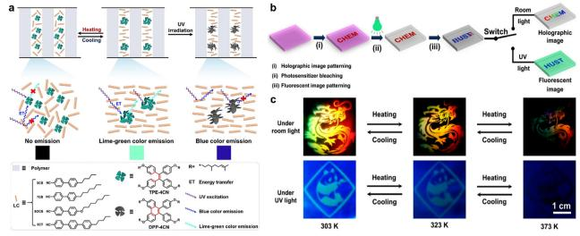
Fig. 7 Liquid crystal (LC)/AlEgen system for patterning crosstalk-free images. (a) Synergistic mechanism for obtaining a holographic pattern and fluorescent pattern in the LC/AlEgen system. (b) Coding procedure for the holographic and fluorescent images. (c) Cooperative-thermoresponse behaviors of the holographic and fluorescent images under room light and UV light, respectively.<sup>71</sup> Reprinted with permission from ref. 71 (Copyright 2020 John Wiley and Sons).
