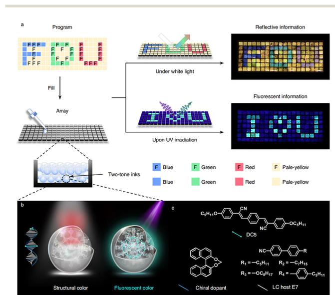
Fig. 6 Geminate labels carrying two distinct kinds of information under white and UV light, respectively. (a) Schematic illustration of a geminate label with two different information items of an "FDU" reflective pattern and an "I♥U" fluorescent pattern. (b) Chemical structures of the materials used to prepare the FCLC mixtures, which show structural color under white light and fluorescent color under UV light.<sup>69</sup> Reprinted with permission from ref. 69 (Copyright 2021 Springer).
