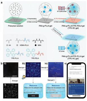
Fig. 13 Multi-level information encryption/decryption based on programmable crystal phases in florescent hydrogels. (a) Designs of PAA-g-PLLA gel, TPE-SC gel and TPE-HC gel. (b) Image showing the complicated QR code with HC and SC crystal phases, exhibiting multi-level encryption/ decryption under UV irradiation and solvent replacement. 92 Reprinted with permission from ref. 92 (Copyright 2023 John Wiley and Sons).
