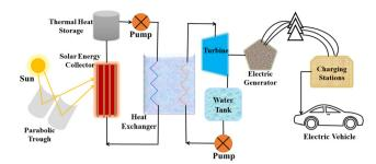
Fig. 5 Basic components of a concentrated solar power plant for the storage of thermal energy.
