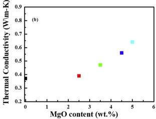
Fig. 20 Experimental data showing the thermal conductivity of NaNO<sub>3</sub>-KNO<sub>3</sub> (a) improves with the addition of MgO at different mass concentrations (2.5%, 3.5%, 4.5% and 5%) with temperature, and (b) the increasing thermal conductivity at different concentrations. Adapted from ref. 35, with permission from Elsevier, Copyright 2020.
