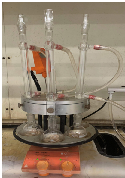
Chart 1 Transesterification reaction under water-cooled reflux in Radley Carousel reactor.
