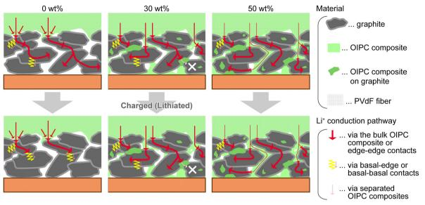
Fig. 11 Role of OIPC in the solid-state electrodes. Mixing OIPC with graphite anode promotes Li<sup>+</sup> conduction and electrochemical reaction in the electrode layer. Reprinted from ref. 115 with permission
