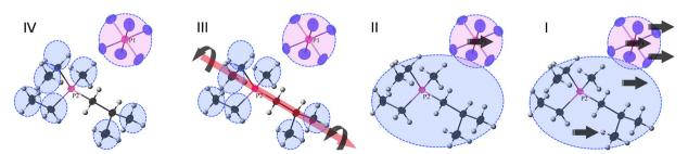
Fig. 7 Schematic of molecular motions in different phases (IV to I) of 26f with increasing temperature. Phase IV, only the methyl and ethyl groups of the cation are rotating, but the anion is tumbling (on the NMR time scale); phase III, the whole cation can rotate around one axis, and the anion continues tumbling; phase II, the whole cation can tumble, and the anion both tumbles and diffuses; phase I, both the cation and the anion can diffuse. Reprinted from ref. 33 with permission.
