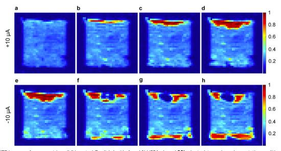
Fig. 6 <sup>1</sup>H SPRITE images of a symmetric cell (Li coated Cu disks) with 4 mol % LiFSA-doped **28b** electrolyte under galvanostatic conditions. (a) Initial cell then continuous application of +10 µA for (b) 17 h, (c) 34 h, and (d) 51 h; and reversed polarity (-10 µA) for the same cell for (e) 6 h, (f) 40 h, (g) 57 h, and (h) 77 h. Reprinted from ref. 69 with permission
