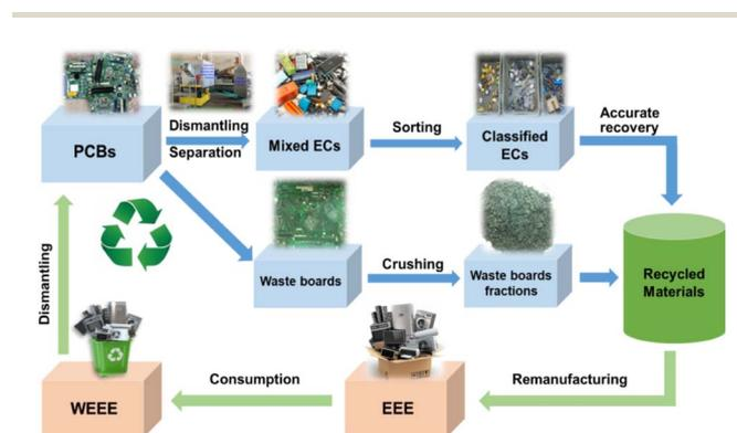
Fig. 3 Recycling flow chart of a PCB in WEEE.<sup>71</sup>
