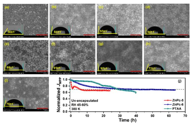
Fig. 8 Surface SEM image of (a) perovskite, (b) ZnPc-1, (c) ZnPc-2, (d) CuPc-3, (e) CuPc-4, (f) ZnPc-5, (g) ZnPc-6, (h) CuPc-7, and (i) CuPc-8 deposited on perovskite. Inset: Corresponding water contact angle. The red lines represent the 1 µm scale bar, and (j) the normalized current density of continuous maximum power point (MPP) tracking for unencapsulated PSCs based on ZnPc-5, ZnPc-6, and pristine PTAA as HTMs under atmospheric conditions (RH 45-65%, 300 K).
