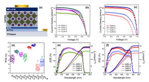
Fig. 6 Proposed device architecture: fluorine-doped tin oxide (FTO)/bl-TiO<sub>2</sub>/SnO<sub>2</sub>/perovskite/MPc/Au (a), J-V curves of the device using (b) symmetric MPcs and (c) asymmetric MPcs, (d) statistical PCE of PSCs with different MPc-HTMs, corresponding IPCE and integrated current density (J<sub>int</sub>) of the device with (e) symmetric MPcs and, (f) asymmetric MPcs
