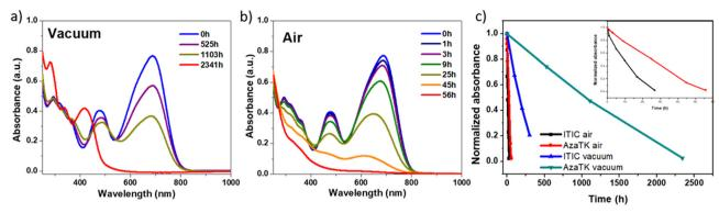
Fig. 6 Absorbance spectra of the evolution of the AzaTk molecule under constant illumination using simulated AM1.5 light in (a) absence of oxygen (vacuum) and (b) presence of oxygen (air). (c) degradation kinetics of both mechanism of AzaTk compared to reference ITIC molecule.
