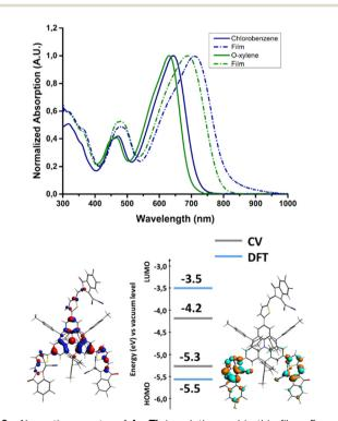
Absorption spectra of AzaTk in solution and in thin films. Energy levels and electron density of the HOMO (left) and LUMO (right) of AzaTk obtained by cyclic voltammetry and DFT calculations
