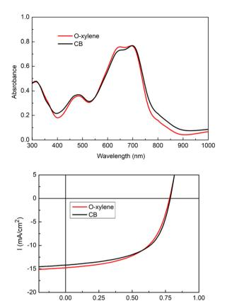
Fig. 3 Absorption spectra and I-V curves of PTB7-Th:AzaTk blend film deposited from o-xylene and chlorobenzene solutions.
