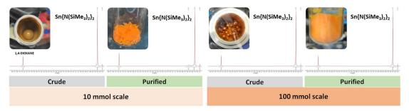
Fig. 2 Side-by-side comparison of the 10 and 100 mmol scale reactions (left and right, respectively) for the synthesis of  $Sn\{N(SiMe_3)_2\}_2$  (2). The inserts display the crude product obtained in 10 mL and the 250 mL stainless steel jars, and the resulting isolated product stored in a 20 mL vial and a 100 mL Schlenk tube for the small and large scales, respectively. See ESI† for expanded NMRs.
